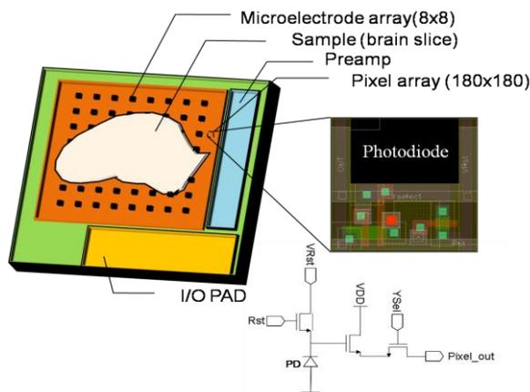
Fig. 1. Schematic representation of Multi-electrode Array Coupled CMOS image sensor (MARC sensor) for *in vitro* electrophysiology.
