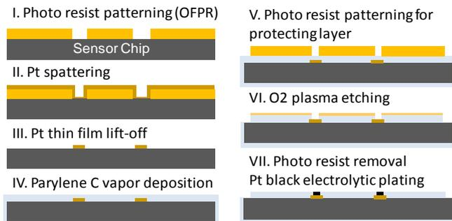
Fig. 3. Schematic representation of Pt black electrode fabrication process
