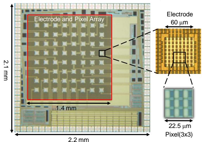
Fig. 2. Microscopic image of MARC sensor, magnified images of single electrode and 3 x 3 pixel array. Multi-electrode array and pixel array were fabricated on the same plane on the sensor chip.
