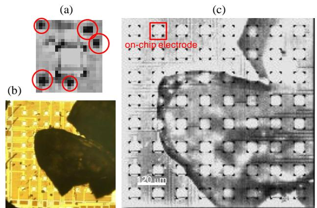
Fig. 5. Functional validation of MARC sensor by imaging biological sample. (a) Captured image of micro beads; the center of the image is on-chip electrode and the diameter of micro bead is 20  $\mu\text{m}$ . (b) Microscopic image of mouse brain slice mounted on MARC sensor. (c) Captured image of mouse hippocampus slice, the on-chip electrode size is 60  $\mu\text{m}$ . (bar = 120  $\mu\text{m}$ )
