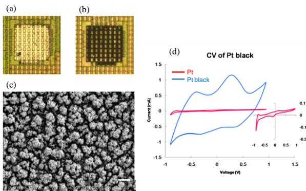
Fig. 4. Evaluation on Pt black electrode. (a) Pt layer on MARC sensor's on-chip electrode. (b) Pt black on MARC sensor's on-chip electrode. (c) SEM observation of Pt black sample electrode (bar = 5  $\mu\text{m}$ ). (d) Cyclic voltammogram of Pt black and Pt (inset) sample electrodes.
