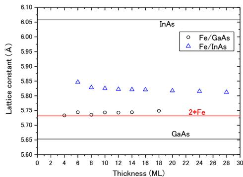
Fig. 2. Changes in lattice constant of Fe/GaAs(001) and Fe/InAs(001) along [010] direction as a function of Fe thickness.
