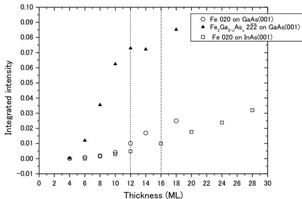
Fig. 3 the changes in the integrated intensity of the 020 diffraction of Fe on GaAs(001), the  $\bar{2}\bar{2}\bar{2}$  diffraction of  $\text{Fe}_3\text{Ga}_{2-x}\text{As}_x$  on GaAs(001) and the 020 diffraction of Fe on InAs(001) as a function of the Fe thickness.
