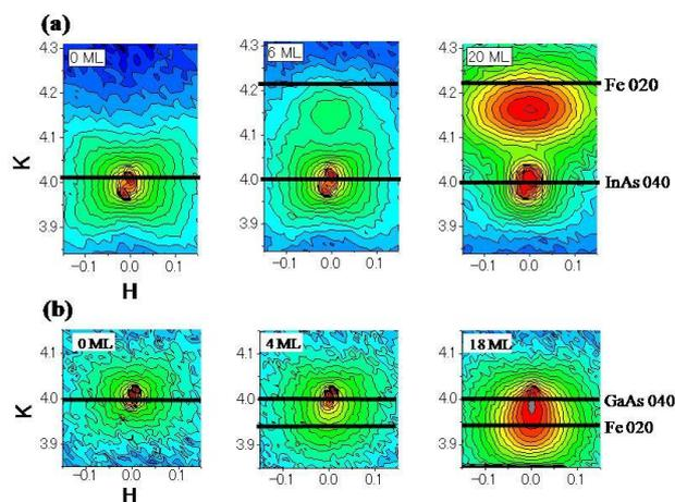
Fig. 1. Reciprocal space maps of InAs(a) and GaAs(b) 040 diffraction at varying Fe thickness.
