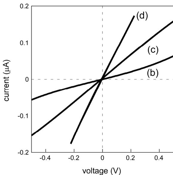
Fig. 2 Current-voltage curves of ZnO NCs. The curves (b)–(d) were measured for the structures presented in Figs. 1(b)–1(d), respectively.
