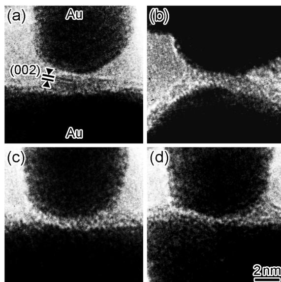
Fig. 1 High-resolution images of ZnO NCs. (a) Before applying bias voltage, NCs in (b)–(d) show conductances of  $2.4 \times 10^{-3}G_0$ ,  $4.4 \times 10^{-3}G_0$  and  $9.9 \times 10^{-3}G_0$ , respectively.
