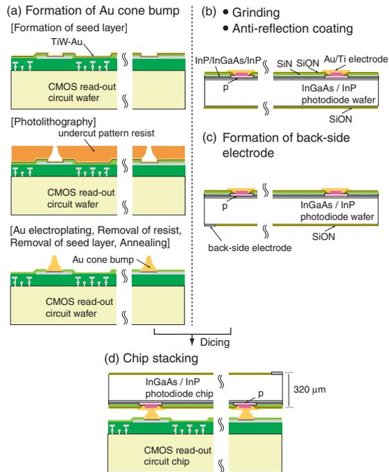
**Fig. 2:** Process flow of the near-infrared image sensor.
