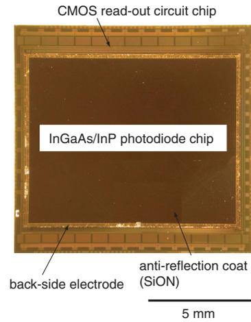
**Fig. 4:** Optical micrograph of the near-infrared image sensor. The InGaAs/InP photodiode chip is stacked onto the CMOS read-out circuit chip by Au cone bumps.
