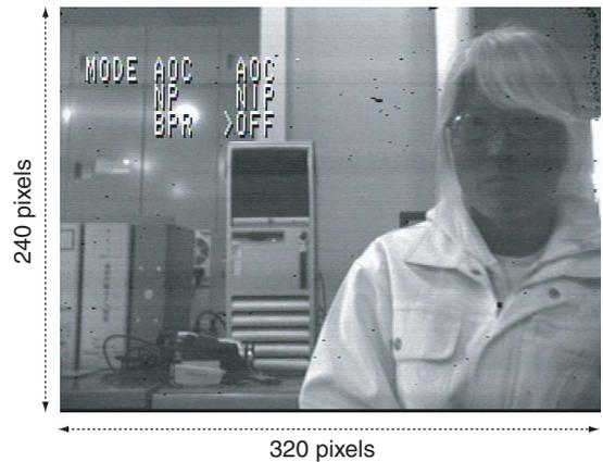
**Fig. 6:** Example of image frames obtained using the near-infrared image sensor. The pixel operability of the image sensor was 99.2%. (number of normal pixels = 76,174, number of defects = 626). No cooling was applied.
