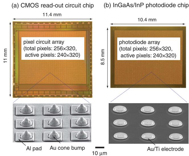
**Fig. 3:** Optical micrographs of the CMOS read-out circuit chip and the InGaAs/InP photodiode chip.
