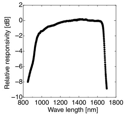
**Fig. 5:** Relative responsivity of the InGaAs/InP photodiode. The maximum relative responsivity was observed at wavelength of 1320–1550 nm.
