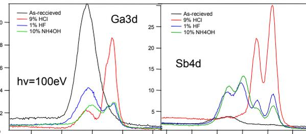
Fig. 4: Effectiveness of (1) 9% HCl (2) 1% HF (3) 10% NH4OH clean in removing  $\text{GaO}_x$  &  $\text{SbO}_x$  is studied using SRPES
