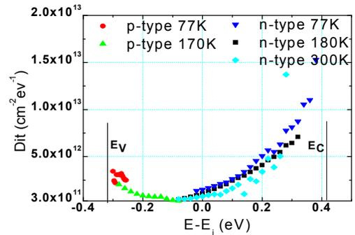
Fig. 10 : Dit distribution is calculated across the bandgap using conductance method. Mid bandgap Dit of  $3 \times 10^{11} \text{ cm}^{-2} \text{ eV}^{-1}$  is achieved.
