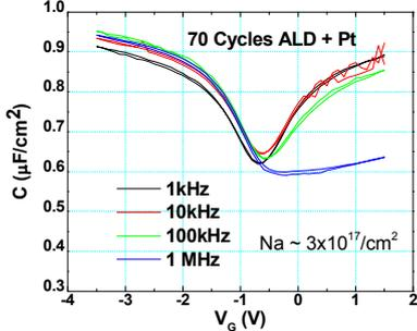
Fig. 9 : Measured CV's from 1kHz-1MHz on p-type (left) & n-type (right) GaSb at 300K.
