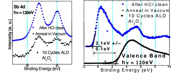
Fig. 6: VBO of  $\text{Al}_2\text{O}_3$  on GaSb is calculated taking the difference in the valence band spectrum (right) Sb 4d peak from the substrate (left) is used for alignment.
