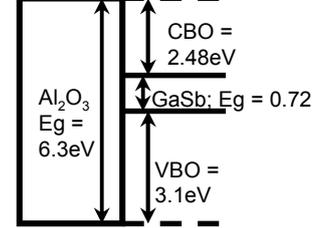
Fig. 8 : Band diagram for  $\text{Al}_2\text{O}_3$  on GaSb.
