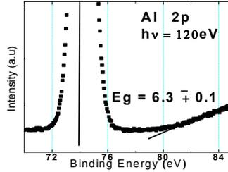
Fig. 7 : Bandgap is calculated from the Al 2p loss spectrum [4].
