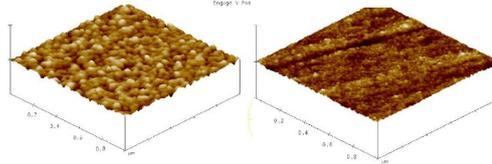
Fig. 2: Tapping mode AFM image of a GaSb left exposed in air for a long time shows (left) RMS roughness = 4.014nm; after HCl Clean + 10 cycles ALD (right) RMS = 0.727nm
