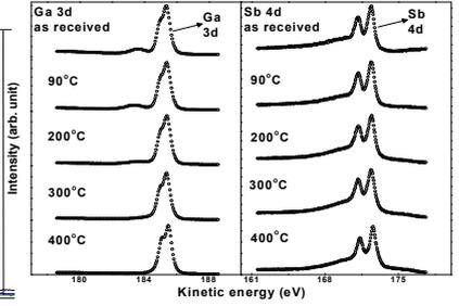
Fig. 5: Cleaning in HCl followed by annealing till 400°C renders a surface free of native oxides.
