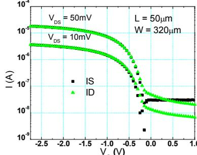
Fig. 13:  $I_D-V_G$  characteristics on the fabricated transistor.
