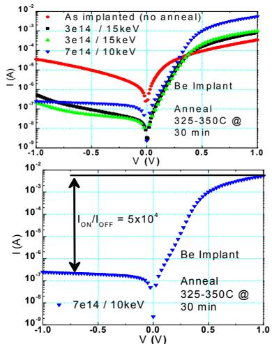
Fig. 11: Optimization of diode using different implant conditions (top)  $I_{ON}/I_{OFF}$  of  $5 \times 10^4$  was achieved (bottom)
