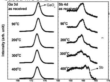
Fig. 3:  $\text{GaO}_x$  shows little desorption till 400°C during anneal under vacuum.
