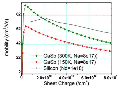
Fig. 14: Hole mobility vs. sheet charge at 300K and 150K calculated from the  $I_D-V_G$  @ 10meV &  $C_{GC}$  measured from the split CV measured.
