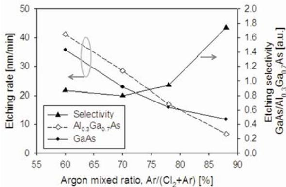
Fig. 3 Etching rates of GaAs and Al<sub>0.3</sub>Ga<sub>0.7</sub>As by NBE with different Ar mixed ratio gas and the etching selectivity of GaAs/Al<sub>0.3</sub>Ga<sub>0.7</sub>As.
