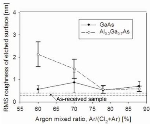
Fig. 2 RMS etched surface roughness of GaAs and Al<sub>0.3</sub>Ga<sub>0.7</sub>As by NBE with different Ar mixed ratio gas.
