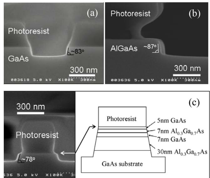
Fig. 4 SEM images of etched profiles of (a) GaAs and (b) Al<sub>0.3</sub>Ga<sub>0.7</sub>As by 78% Ar mixed ratio NBE.
