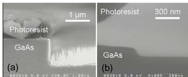
Fig. 1 SEM images of GaAs etched results by neutral beam with (a) 40 sccm Cl<sub>2</sub> reaction gas and (b) 9 sccm (22%) Cl<sub>2</sub> and 31 sccm (78%) Ar mixed gas.
