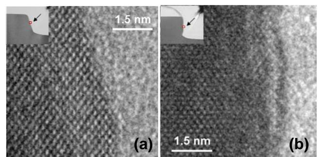
Fig. 5 HRTEM images of GaAs sidewall surfaces etched by (a) NBE and (b) RIE.
