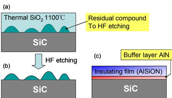
Fig. 2. Surface of thermal oxidized SiC (a) before and (b) after HF etching, and (c) the structure of the inserted AlN.
