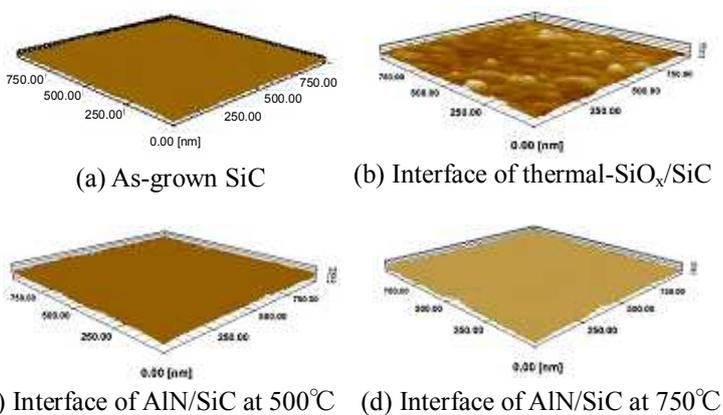
Fig. 3. AFM images of the SiC surface after HF wet treatment.
