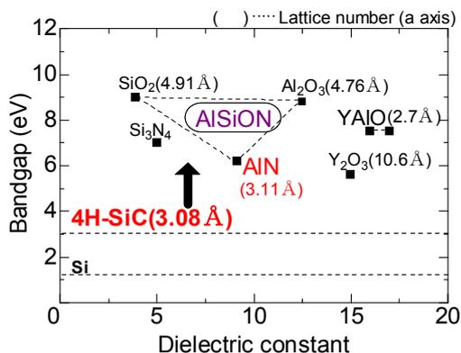
Fig. 1. Bandgap and dielectric constant of various insulating films.
