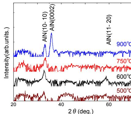
Fig. 4. XRD spectra of AlN films deposited on SiC at various temperatures.
