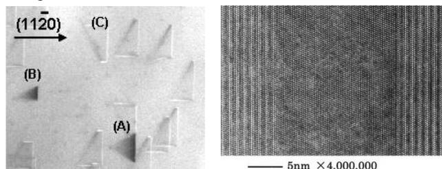
Figure 3 PL topographic image of Non-radiative SF Figure 4 Cross sectional TEM of non-radiative SF
