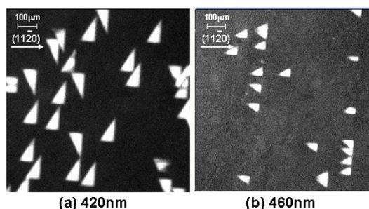
Figure 2 PL topographic imaging of SiC epitaxial layer including some types of SFs at the same spot
