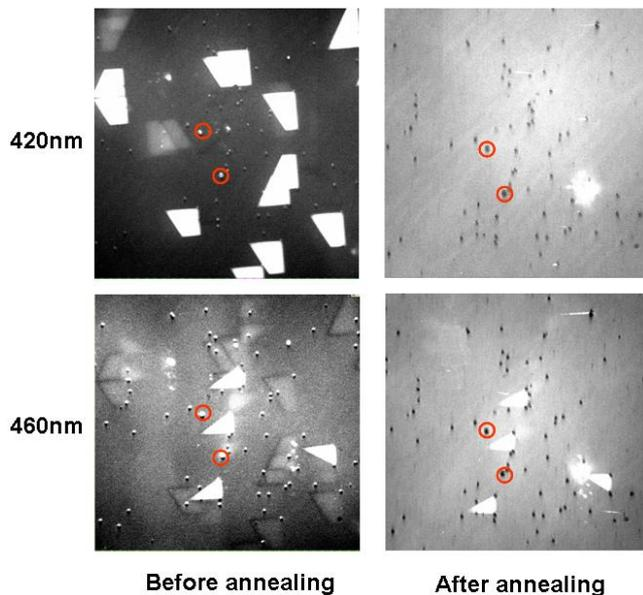
Figure 5 PL topographic patterns before and after annealing process
