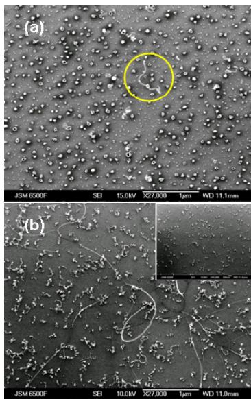
Fig. 1 FE-SEM images after CNT growth from a Ge film on SiO<sub>2</sub> substrate without (a) and with Ar annealing (b).
