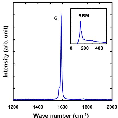
Fig. 2 Raman spectra of CNTs grown from a Ge film on SiO<sub>2</sub> substrate. The inset shows radial breathing mode, indicating that SWNTs are present.
