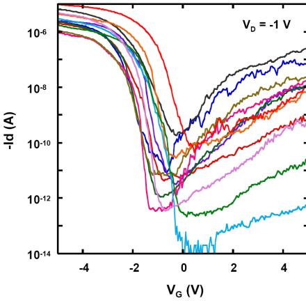
Fig. 3 The sub-threshold characteristics of Pd contacted back gate CNTFETs ( $L_G = 2.0 \mu\text{m}$ ) with  $\text{SiO}_2$  gate insulators.
