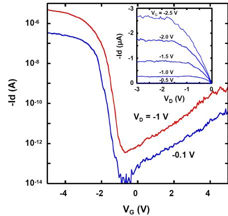
Fig. 4 I-V characteristics of a Pd contacted CNTFET ( $L_G = 2.0 \mu\text{m}$ ). Sub-threshold characteristics for  $V_D = -0.1$  and  $-1.0 \text{ V}$  and output characteristics for  $V_G = -0.5, -1.0, -1.5, -2.0, -2.5 \text{ V}$ .
