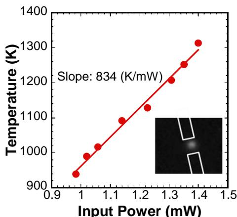
Fig. 2 Input electrical power dependence of the steady state temperature for the suspended MWNT.
