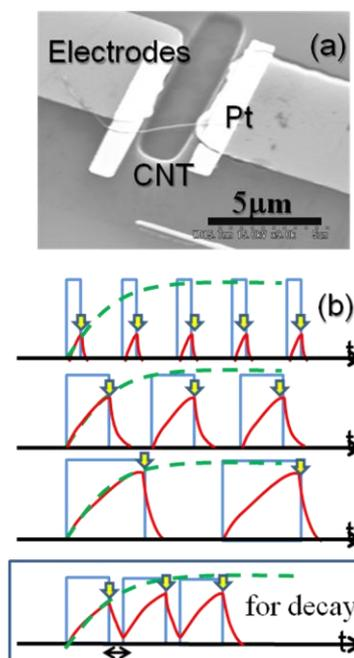
Fig. 1 (a) SEM image of the suspended MWNT after Pt deposition by e-beam lithography. (b) Timing chart of the pulsed voltage measurement for transient thermal response
