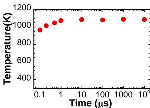
Fig. 3 Pulse width dependence of the temperature corresponding to the rising edge property.
