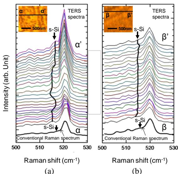
Fig. 4 TERS spectra obtained from strained-Si layers on quadruple-Si<sub>1-x</sub>Ge<sub>x</sub>-layer buffers formed by (a) GS-MBE, and (b) our sputter epitaxy. The TERS spectra were measured at points along the  $\alpha$ - $\alpha'$  and  $\beta$ - $\beta'$  lines (1500 nm) indicated in the inserted AFM images.
