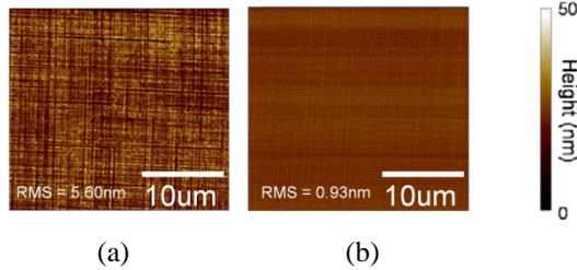
Fig. 3. Wide-area (30 x 30 μm) AFM topographies obtained from the surfaces of strained-Si on quadruple-Si<sub>1-x</sub>Ge<sub>x</sub>-layer buffers formed by (a) GS-MBE and (b) our sputter epitaxy.
