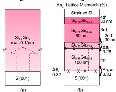
Fig. 1 Strain-relief relaxed buffers: (a) a commonly used thick  $\text{Si}_{1-x}\text{Ge}_x$  graded buffer, (b) our proposed quadruple- $\text{Si}_{1-x}\text{Ge}_x$  layer buffer and strained Si grown on it. [1]
