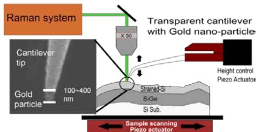
Fig.2 Schematic of AFM-TERS system
