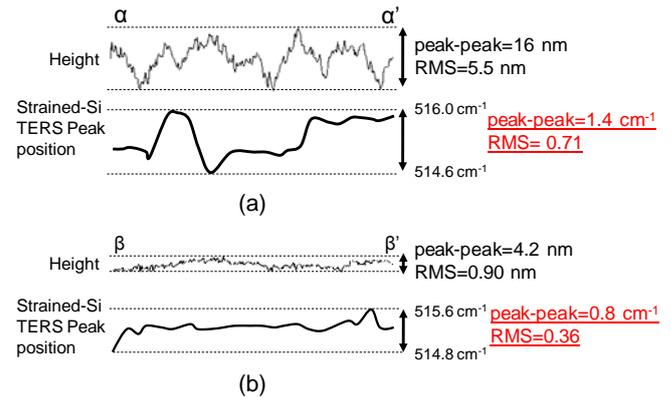
Fig. 5 AFM surface undulation traces and s-Si TERS peak positions measured along the 1500-nm  $\alpha$ - $\alpha'$  and  $\beta$ - $\beta'$  lines indicated in the AFM images inserted in Figs. 4(a) and (b) for the samples formed by (a) GS-MBE and (b) our sputter epitaxy.
