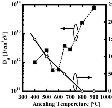
Fig. 4  $D_{it}$  and Hysteresis width of deferent PDA temperature.
