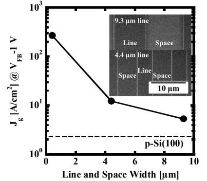
Fig. 7 Line width dependence of J-V characteristics.
