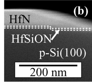
Fig. 2 (a) Schematic and (b) SEM image of fabricated 3D MIS diode.
