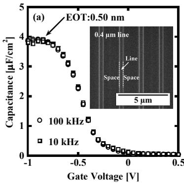
Fig. 6 (a) C-V and (b) J-V characteristics of HfN/HfSiON gate stacks on 3D Si structures.
