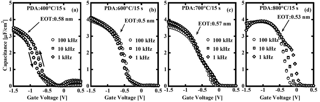
Fig. 3 PDA temperature dependence of C-V characteristics of planar HfN/HfSiON/p-Si(100) gate stacks. PDA temperatures are (a) 400°C, (b) 600°C, (c) 700°C, and (d) 800°C.
