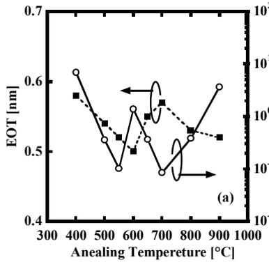
Fig. 5 (a) PDA temperature dependence of EOT and leakage current at  $V_{FB}-1$  V (b) EOT versus current densities plot.
