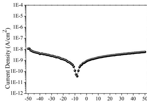
Fig. 2. Leakage current density of MIM with mr-UVCur06 as a dielectric. The voltage was varied from –50 to 50 V.
