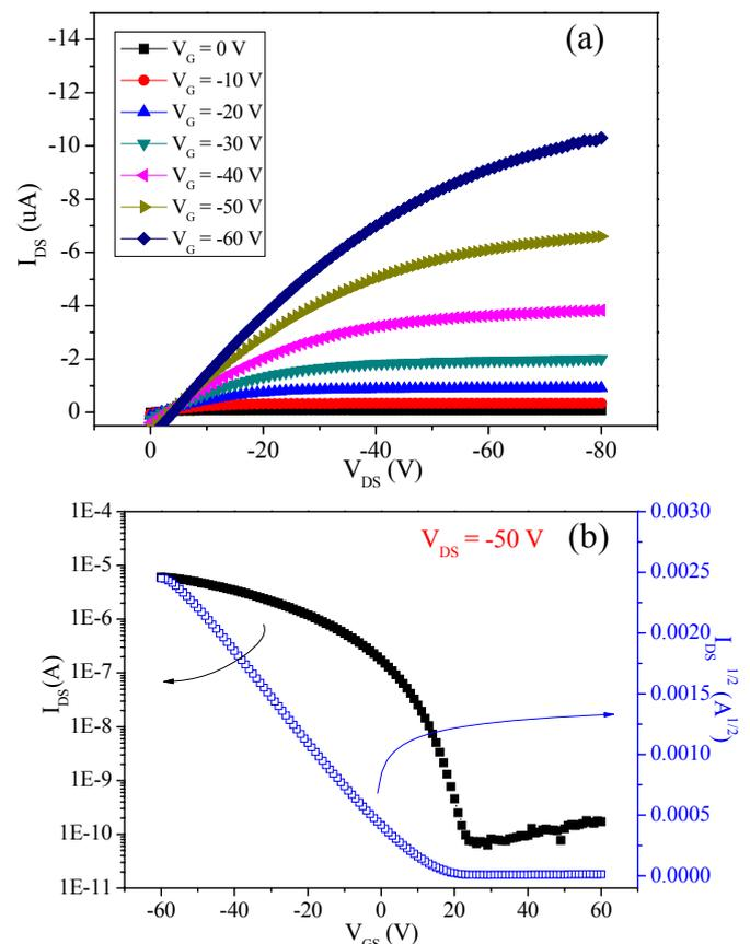
Fig. 4(a). The output characteristics of  $I_{DS}$  versus  $V_{DS}$  of OTFTs. (b) The transfer characteristics of  $I_{DS}$  versus  $V_{GS}$  and the square root of the  $I_{DS}$  versus  $V_{GS}$  of OTFTs with mr-UVCur06 as gate dielectric.
