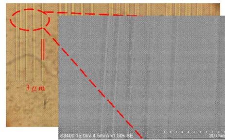
Fig. 3. Optical microscopy image and cross-sectional SEM image for a pattern with 3 μm line/space resolution.
