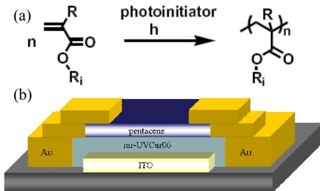
Fig. 1. (a) Free-radical polymerisation of (meth)acrylates initiated by UV exposure (acrylates R=H, methacrylates R=CH<sub>3</sub>, Ri various functional groups). (b) Schematic cross section of a pentacene-base OTFT with low-temperature processable photosensitive polymerization.
