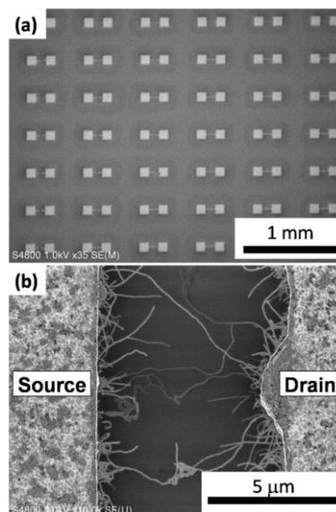
Fig.1 Typical SEM image of an array of SWNT-FETs (a) and nanotube channel between source/drain electrodes (b).
