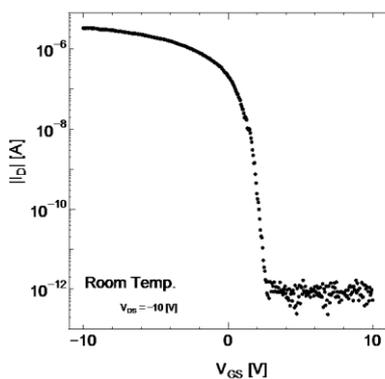
Fig.2 Transfer characteristics of the fabricated device with electrode width of 40  $\mu\text{m}$  operated at room temperature.  $V_{DS} = -10$  V.
