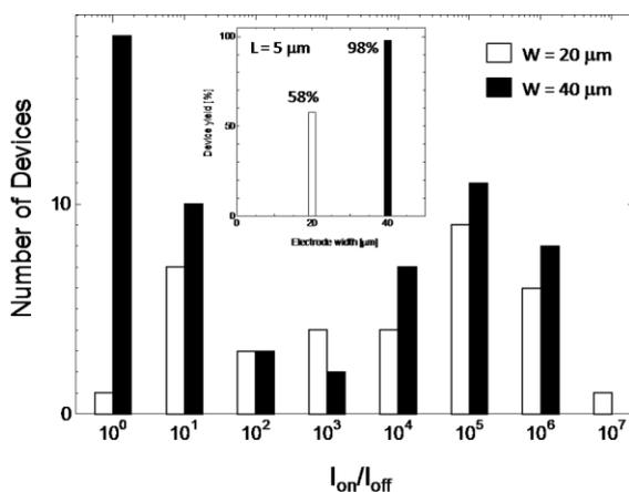
Fig.3 Histogram of  $I_{on}/I_{off}$  ratio of the fabricated devices. The open and solid bar means electrode width of 20  $\mu\text{m}$  and 40  $\mu\text{m}$ , respectively. The inset shows the device yield when channel length is 5  $\mu\text{m}$ .
