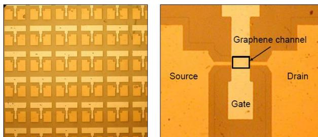
Fig. 1 Optical microscope image of graphene FET arrays.
