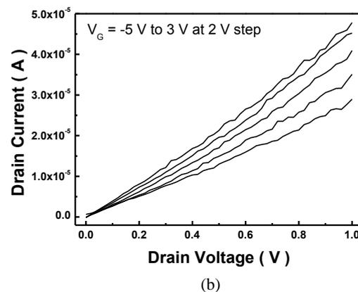
Fig. 4 Electrical characteristics of the epitaxial graphene FET using the polymer gate dielectric. (a)  $I_d$ - $V_g$  characteristics, (b)  $I_d$ - $V_d$  characteristics.
