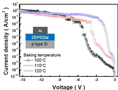
Fig. 2 I-V characteristics of MIS capacitors for three baking temperatures employed in the polymer fabrication process.
