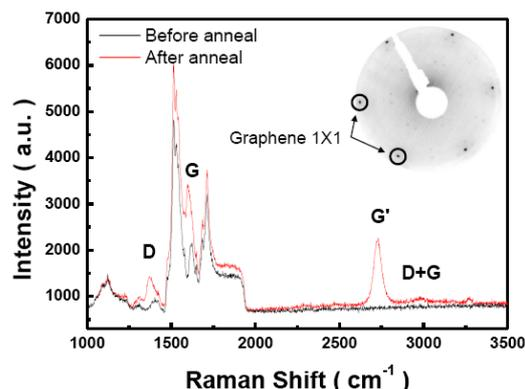
Fig. 3 Raman spectra of the SiC substrate before and after the graphitization anneal. Inset is a LEED pattern of the annealed 6H SiC substrate, indicating formation of epitaxial graphene.
