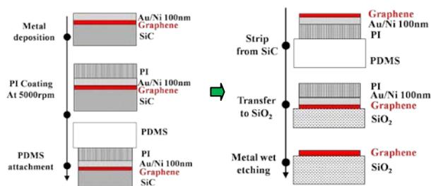
Fig.1 Schematic flow and picture of samples showing the process of graphene transfer from the SiC substrate
