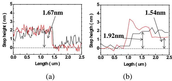
Fig.4 Step heights of graphene transferred on SiO<sub>2</sub>, measured by Atomic Force Microscope(AFM); (a) Au, (b) Ni
