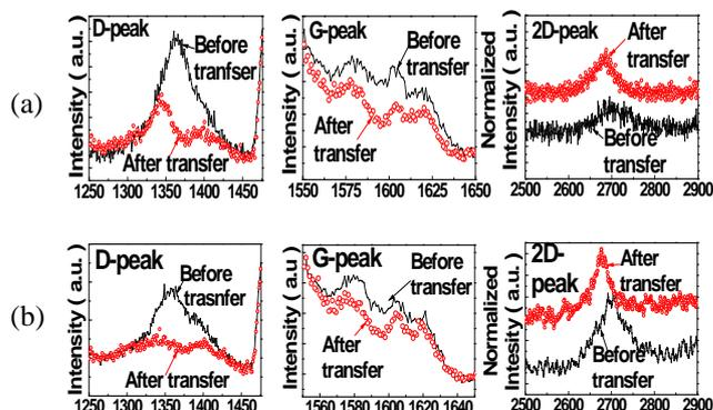
Fig.3 Raman Spectrum of graphitized SiC ; (a) Au (before / after ) (b)Ni(before/after) the graphene transfer
