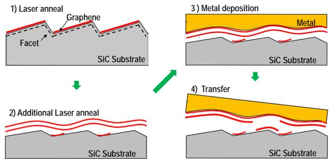
Fig.6 Schematic diagram of graphene transfer from a graphitized SiC surface using a metal thin film adhesion layer
