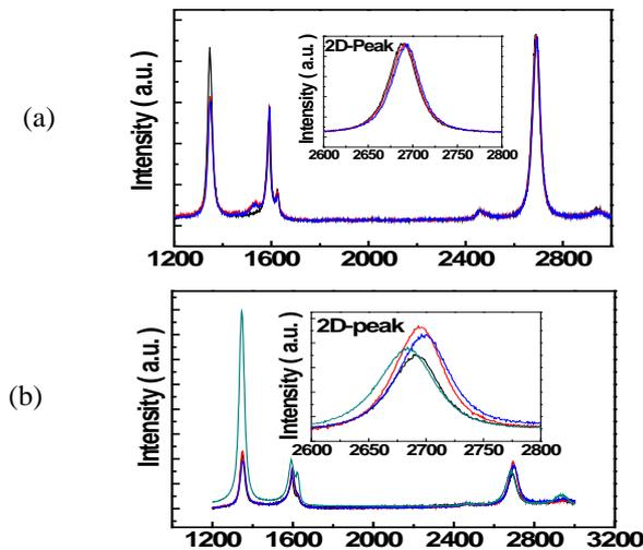
Fig.5 Raman Spectrum of graphene films transferred to SiO<sub>2</sub> 300nm/Si substrate; (a) Au, (b) Ni
