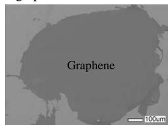
Fig.2 SEM photograph of transferred graphene on SiO<sub>2</sub>
