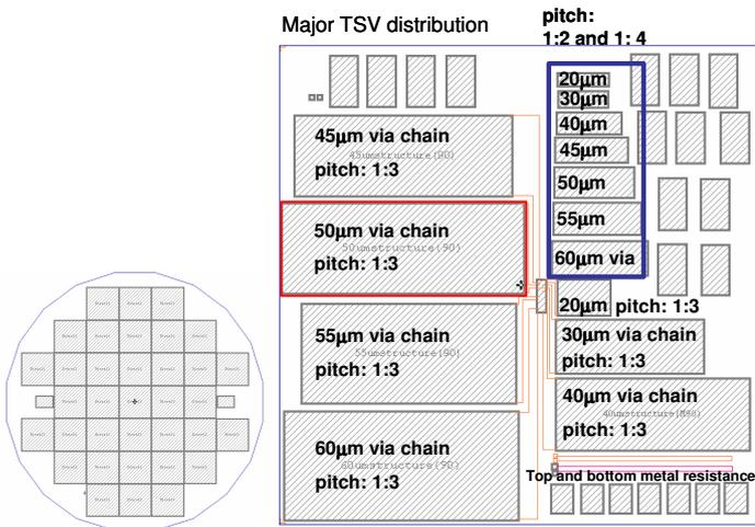
Fig. 1. Schematic illustration of a TSV test chip wafer map and major TSV distribution maps in individual test chips used in this study.
