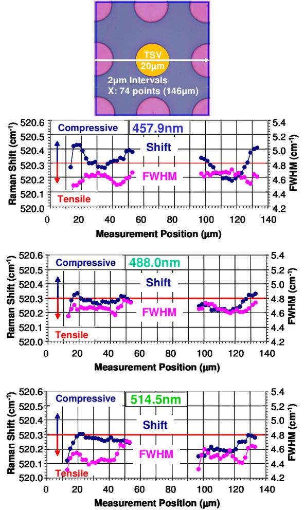
Fig. 3. Multi-wavelength line scan summary of Raman shift and FWHM of Si region between 20µm diameter Cu filled TSVs.
