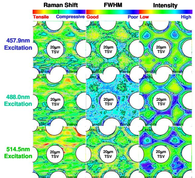
Fig. 4. Multi-wavelength area map summary of Raman shift, FWHM, and intensity in Si surrounded by 20µm diameter Cu filled TSV matrix.
