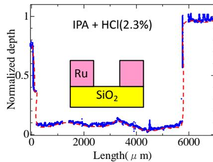
Fig.6 Step profile of the etched pattern.
