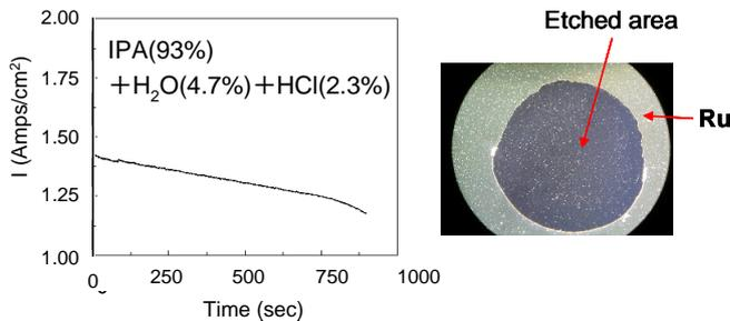
Fig. 4 (a) Time dependence of corrosion currents, and (b) etched pattern by IPA based HCl solution.
