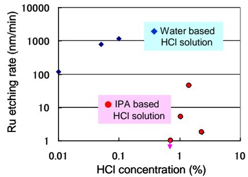
Fig.5 Dependence of Ru etching rates on HCl concentration.
