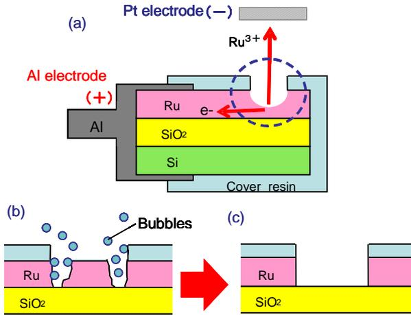
Fig.1 (a) Cross section of Ru sample for this experiment. (b) A conventional etched pattern. (c) An ideal etched pattern.
