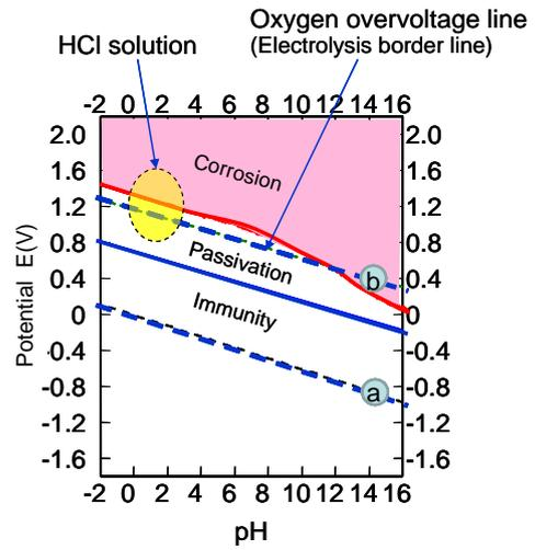
Fig.2 pH-potential diagram of Ru. (Pourbaix Diagram)
