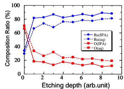
Fig.7 XPS depth profile of composition ratio in the Ru films after electrochemical etching.
