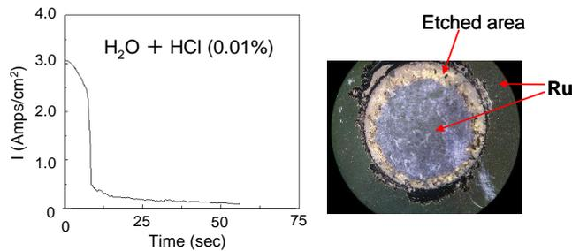
Fig. 3 (a) Time dependence of corrosion currents, and (b) etched pattern by water based HCl solution.
