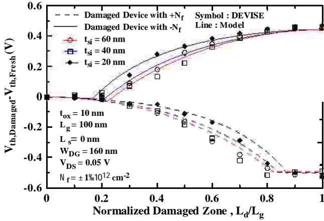
Fig. 2 Threshold voltage degradation versus normalized damaged zone for different diameters of silicon body.
