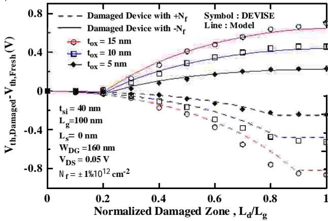
Fig. 3 Threshold voltage degradation versus normalized damaged zone for different oxide thicknesses.
