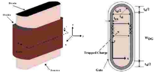
Fig. 1 Schematic of surrounding-gate MOSFETs: (a) three-dimensional device structure, (b) two-dimensional device structure to derive the model. Regions 1, 2, and 3 denote low field region near source, high field region with damage and high field region without damage.
