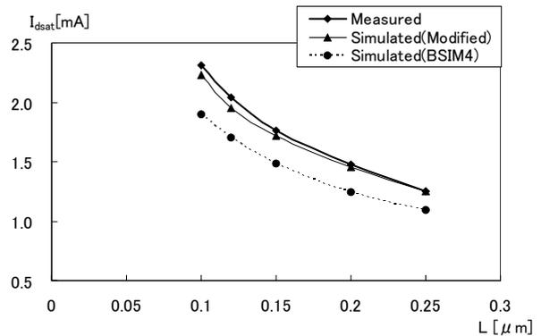
Fig. 4. Saturation current,  $I_{dsat}$ , dependencies on channel length ( $W = 3.0 \text{ } \mu\text{m}$ ). Here,  $I_{dsat}$  was obtained at  $V_{DD} = V_{gs} = 1.0 \text{ V}$  and  $V_b = 0.5 \text{ V}$ .
