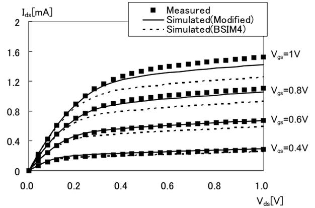
Fig. 3. Characteristic of measured and simulated  $I_{ds}$  versus  $V_{ds}$  at  $V_b = 0.5 \text{ V}$  (forward biased). Gate channel length,  $L$ , and gate channel width,  $W$  are  $90.0 \text{ nm}$  and  $2.0 \text{ } \mu\text{m}$ .
