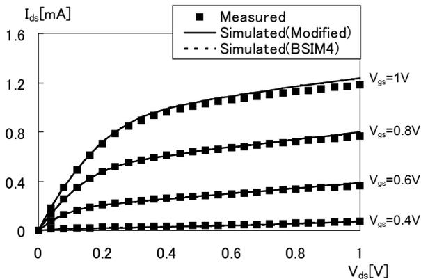
Fig. 2. Characteristic of measured and simulated  $I_{ds}$  versus  $V_{ds}$  at  $V_b = -1.0 \text{ V}$  (reverse biased). Gate channel length,  $L$ , and  $W$  are  $90.0 \text{ nm}$ , and  $2.0 \text{ } \mu\text{m}$ .
