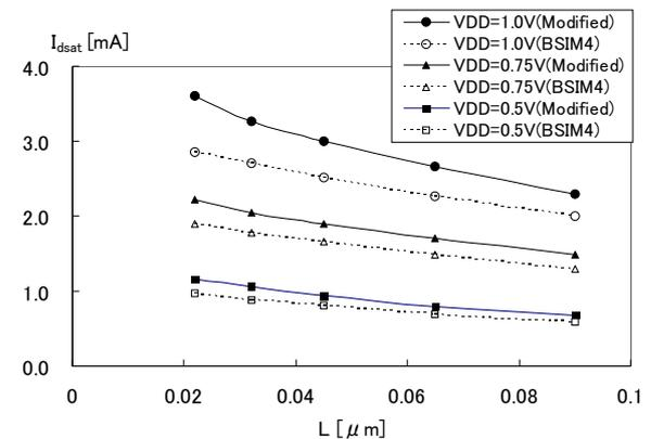
Fig. 5. Predictive simulations for shorter channel length devices ( $W = 3.0 \text{ } \mu\text{m}$ ). Here,  $V_{gs}$  is equals to  $V_{DD}$  and  $V_b$  was fixed to  $0.5 \text{ V}$ . Model parameters were extracted by T-CAD simulations.
