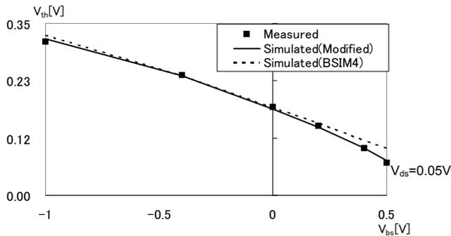
Fig. 1.  $V_{th}$ , dependencies on reverse-to-forward body biases. Here,  $V_{th}$  was adopted by the  $V_{gs}$  at the  $I_{ds}$  of  $100 \text{ nA} \times W/L$ .  $L = 0.25 \text{ } \mu\text{m}$ ,  $W = 3.0 \text{ } \mu\text{m}$ .
