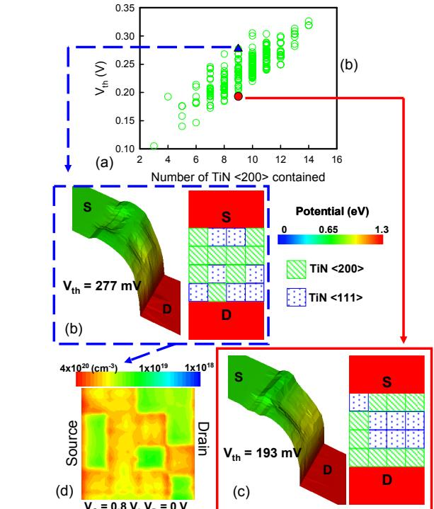
Fig. 4. (a) Threshold voltage distribution as a function of number of TiN  $<200>$  contained for NMOS. The on-state ( $V_G = 0.8 \text{ V}$ ,  $V_D = 0.8 \text{ V}$ ) potential distributions of (b) higher  $V_{th}$  and (c) lower  $V_{th}$ , devices with the same number of TiN  $<200>$ . (d) The charge distribution extracted from (b) at  $V_G = 0.8 \text{ V}$ ,  $V_D = 0 \text{ V}$ .
