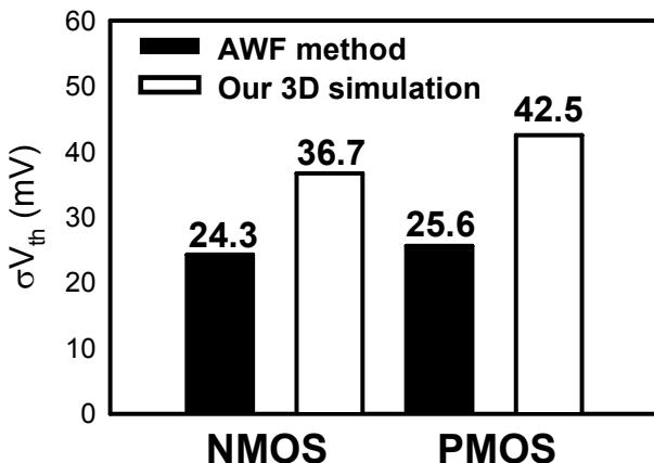
Fig. 3.  $\sigma V_{th}$  comparison between AWF method and our 3D device simulation. AWF method underestimates WKF because it does not reflect the nonuniform surface charge distribution due to the different crystal orientation of nanosized metal grain locally.
