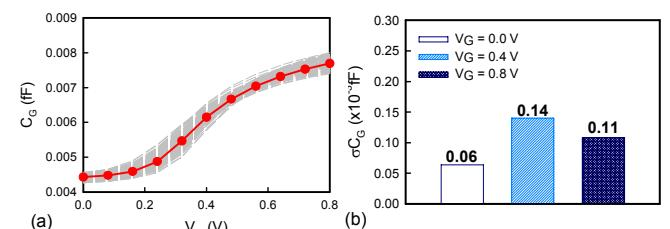
Fig. 5. (a) The WK fluctuated  $C_G$ - $V_G$  curves of NMOS. (b) The summarized  $\sigma C_G$  of device at different gate bias.
