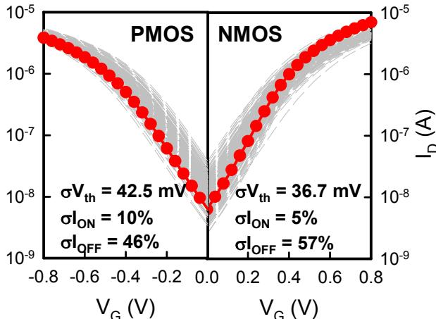
Figure 2. The WK fluctuated  $I_D$ - $V_G$  curves for the tested (a) NMOS (b) and PMOS devices, where the nominal curves with WK of 4.52 eV and 4.76 eV are the red thick symbol lines. The  $\sigma V_{th}$ , and the normalized  $\sigma I_{ON}$  and  $\sigma I_{OFF}$  are listed in the inset.
