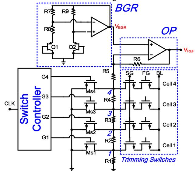
Fig. 2 The complete voltage reference circuit with four trimming switches to fine tune  $V_{\text{REF}}$ .
