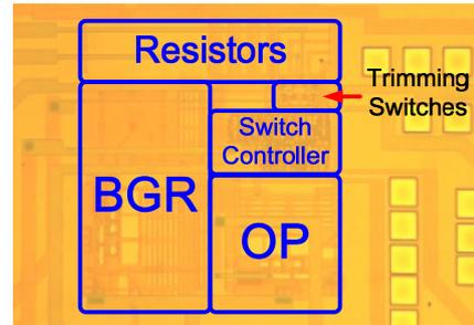
Fig. 3 The chip photograph corresponding to the circuit in Fig. 2 with the trimming switches indicated by the arrow.
