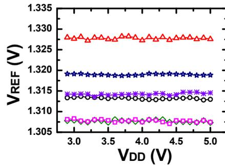
Fig. 4 (b)  $V_{REF}$  versus supply voltages after trimming at  $25^\circ\text{C}$
