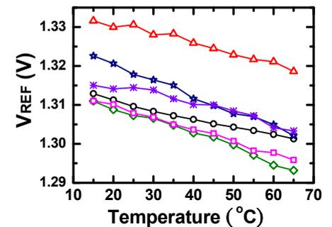
Fig. 5 (b)  $V_{REF}$  versus temperatures after trimming for  $V_{DD}=3.3\text{V}$
