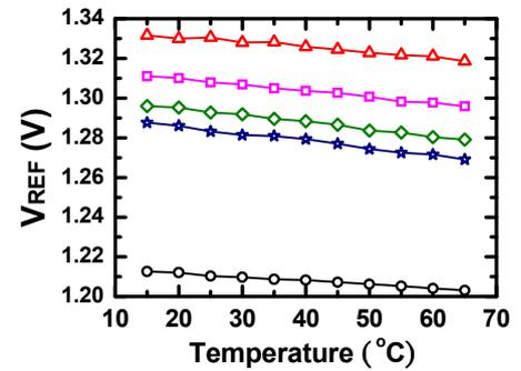
Fig. 5 (a)  $V_{REF}$  versus temperatures before trimming for  $V_{DD}=3.3\text{V}$
