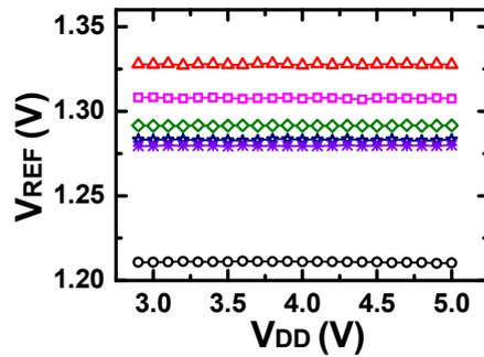
Fig. 4 (a)  $V_{REF}$  versus supply voltages before trimming at  $25^\circ\text{C}$
