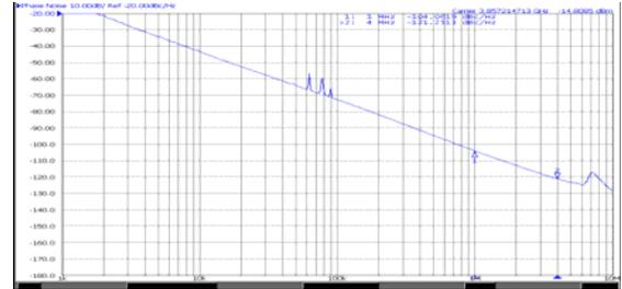
Fig.4. Measured phase noise of proposed DCO at 3.86 GHz oscillating frequency
