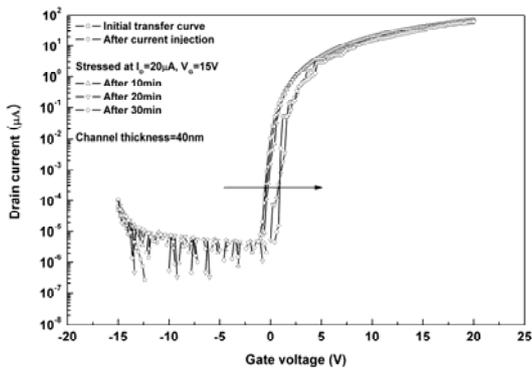
Fig. 3. Transfer characteristics variation for the a-IGZO TFT with 40-nm channel thickness.
