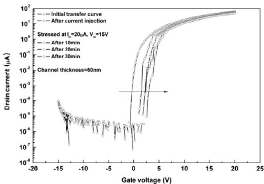
Fig. 4. Transfer characteristics variation for the a-IGZO TFT with 60-nm channel thickness.
