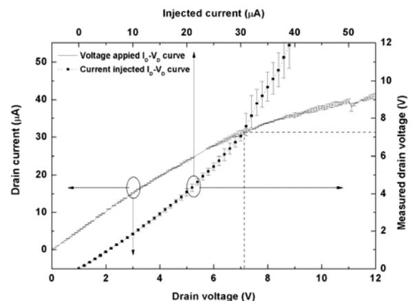
Fig. 2. Comparison between voltage applied  $I_D$ - $V_D$  and current injected  $I_D$ - $V_D$  curves. (a-IGZO thickness = 60 nm and  $V_G = 15$  V.)
