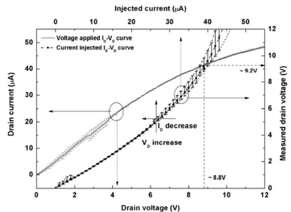
Fig. 1. Comparison between voltage applied  $I_D$ - $V_D$  and current injected  $I_D$ - $V_D$  curves. (a-IGZO thickness = 40 nm and  $V_G = 15$  V.)
