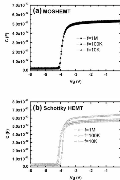
Fig. 2 Typical C-V characteristics of MOSHEMT (oxidized at 450°C)(a) and Schottky HEMT (b) measured at 1MHz, 100kHz and 10kHz
