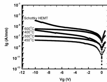
Fig. 1 the gate leakage current of MOSHEMT at different oxidation temperatures and Schottky HEMT as a function of gate voltage
