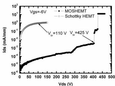
Fig. 5 the breakdown properties of MOSHEMT (oxidized at 450°C) and Schottky HEMT, at pinch-off state
