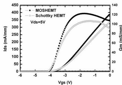
Fig. 4 Measured transfer and transconductance characteristics of the MOSHEMT (oxidized at 450°C) and the Schottky HEMT
