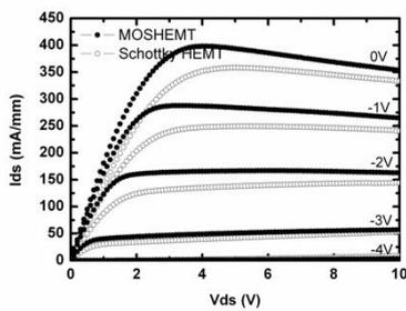
Fig. 3 Measured I-V output characteristics of the MOSHEMT (oxidized at 450°C) and the Schottky HEMT
