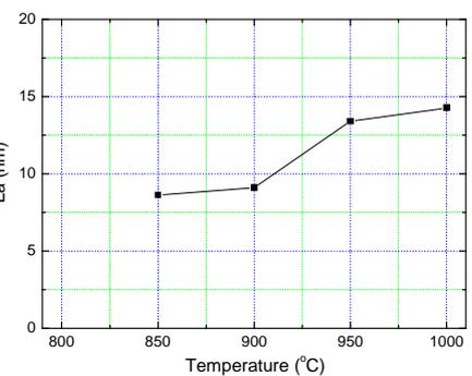
Fig.4 Temperature dependence of the domain size of graphene network (La) on sapphire substrates.
