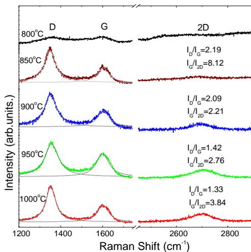
Fig.3 Temperature dependence of Raman spectra of carbon films on sapphire substrates at the 50sccm ethanol gas flow for 15min.
