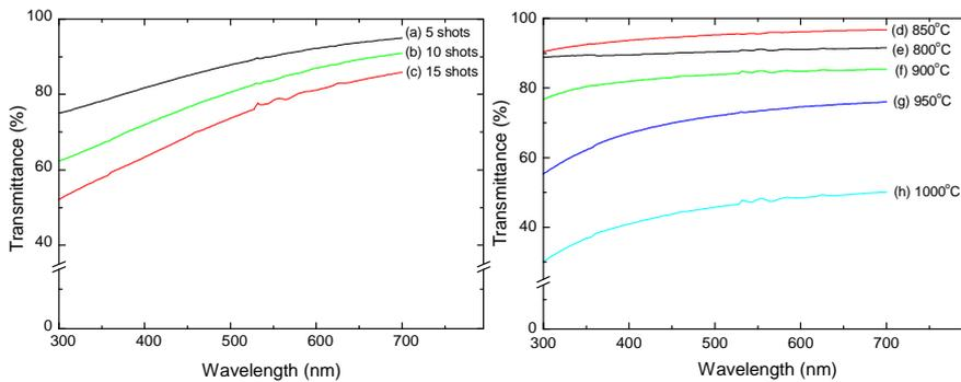
Fig.1 Transmittance spectra of carbon films by DC discharge sputtering on sapphire substrates. Shots represent times of DC discharge flashing.
