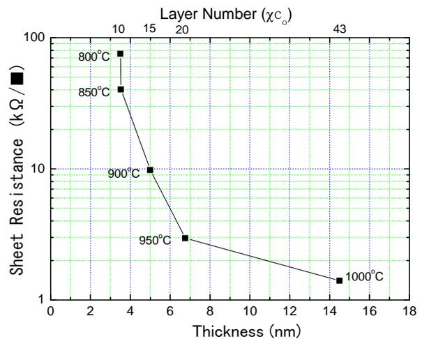
Fig.5 Thickness and number of layers dependence of sheet resistivity of carbon films on sapphire substrates.
