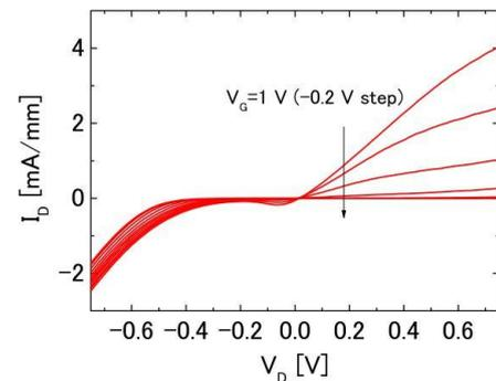
Fig. 5.  $I_D$ - $V_D$  characteristics.
