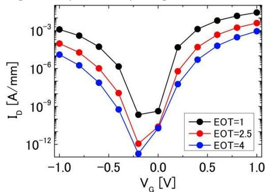
Fig. 1. Simulated  $I_D$ - $V_G$  characteristics.
