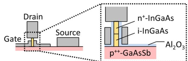
Fig. 2. Fabricated device structure.
