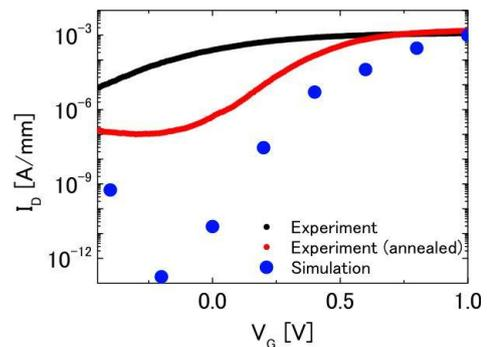
Fig. 6. Comparison between observed characteristics at  $V_D=0.25$  V and simulated characteristics at  $V_D=0.3$  V.
