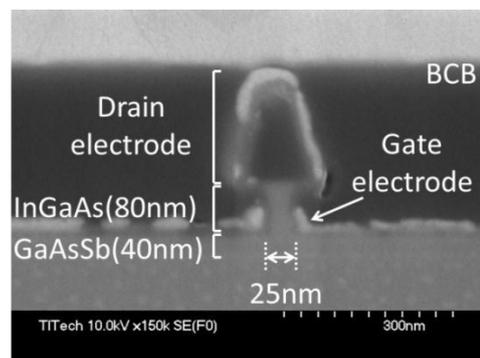
Fig. 3. SEM cross-section image of fabricated device.
