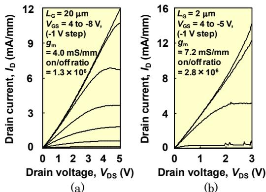
Fig. 2  $I_D$ - $V_{DS}$  characteristics of the fabricated ZnO-TFTs (a) with 20  $\mu$ m-gate-length, (b) with 2  $\mu$ m-gate-length, respectively.
