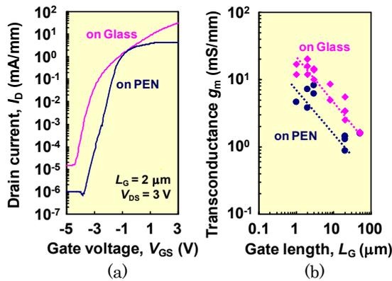
Fig. 3 Comparison of on/off ratio and  $g_m$  in ZnO-TFT between on glass substrate with on PEN substrate. (a) On/off ratio, (b) transconductance,  $g_m$ .
