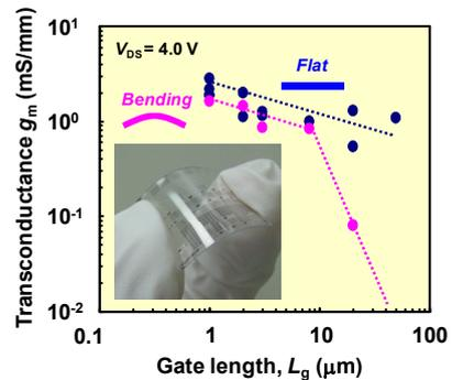
Fig. 5 The  $g_m$ - $L_G$  characteristics of ZnO-TFTs on PEN compared the flat state and bending state.
