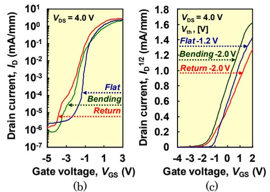
Fig. 4 (a)  $I_D$ - $V_{DS}$  characteristics of the fabricated ZnO-TFTs on a flexible PEN substrate by the different conditions (flat, bending, and return). (b) Transfer characteristics and (c) threshold voltage,  $V_{TH}$  of the fabricated ZnO-TFTs on PEN.
