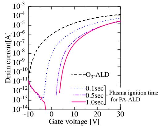
Fig. 4 Transfer characteristics of ZnO TFT with Al<sub>2</sub>O<sub>3</sub> gate insulator.
