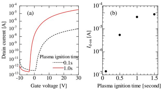
Fig. 3 (a) Transfer characteristics of the ZnO TFTs annealed at 300°C, (b) dependence of  $I_{d,on}$  on plasma ignition time.
