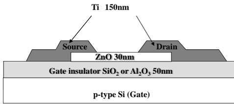
Fig. 2. Schematics of a bottom-gate type TFT
