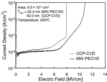
Fig. 3.  $J-E$  characteristics of GaN MOS capacitors with MW-PECVD  $\text{SiO}_2$  and CCP-CVD  $\text{SiO}_2$  at  $200^\circ\text{C}$ .  $\text{SiO}_2$  films were not annealed after deposition. Electric field is defined  $(V_g - V_{FB})/EOT$  ( $V_g$ : gate voltage,  $V_{FB}$ : flatband voltage shift,  $EOT$ : equivalent oxide thickness)
