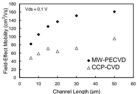
Fig. 8. Field-effect mobility versus channel length of AlGaIn/GaN Hybrid MOS-HFETs with MW-PECVD  $\text{SiO}_2$  and CCP-CVD  $\text{SiO}_2$ .  $\text{SiO}_2$  films were annealed at  $800^\circ\text{C}$  for 30 min after deposition.
