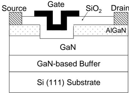
Fig. 1. A schematic cross section of AlGaIn/GaN Hybrid MOS-HFET.
