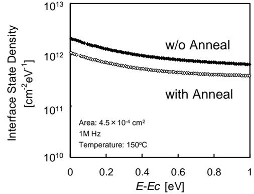
Fig. 5.  $D_{it}$  of GaN MOS capacitors with and without annealing after MW-PECVD  $\text{SiO}_2$  deposition calculated from the  $C-V$  characteristics at  $150^\circ\text{C}$ . (Annealing:  $800^\circ\text{C}$ , 30 min)
