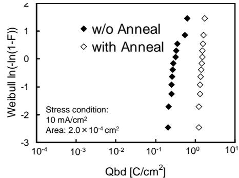
Fig. 6. Charge-to-breakdown  $Q_{bd}$  of GaN MOS capacitors with and without annealing after MW-PECVD  $\text{SiO}_2$  deposition calculated from the  $C-V$  characteristics at  $150^\circ\text{C}$ . (Annealing:  $800^\circ\text{C}$ , 30 min)
