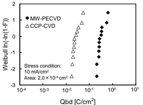
Fig. 4. Charge-to-breakdown  $Q_{bd}$  of GaN MOS capacitors with MW-PECVD  $\text{SiO}_2$  and CCP-CVD  $\text{SiO}_2$ .  $\text{SiO}_2$  films were not annealed after deposition.
