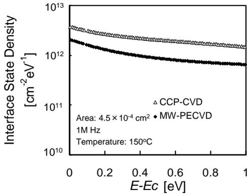
Fig. 2.  $D_{it}$  of GaN MOS capacitors with MW-PECVD  $\text{SiO}_2$  and CCP-CVD  $\text{SiO}_2$  calculated from the  $C-V$  characteristics at  $150^\circ\text{C}$ .  $\text{SiO}_2$  films were not annealed after deposition.
