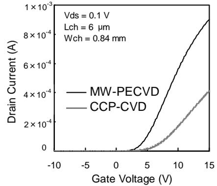
Fig. 7. Transfer characteristics of AlGaIn/GaN Hybrid MOS-HFETs with MW-PECVD  $\text{SiO}_2$  and CCP-CVD  $\text{SiO}_2$ .  $\text{SiO}_2$  films were annealed at  $800^\circ\text{C}$  for 30 min after deposition.
