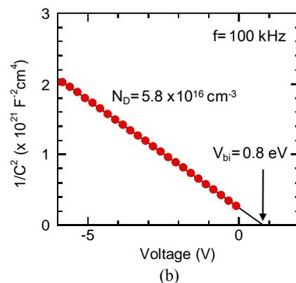
Fig.2 (a) I-V and (b)  $1/C^2$ -V characteristics of the Schottky sample.
