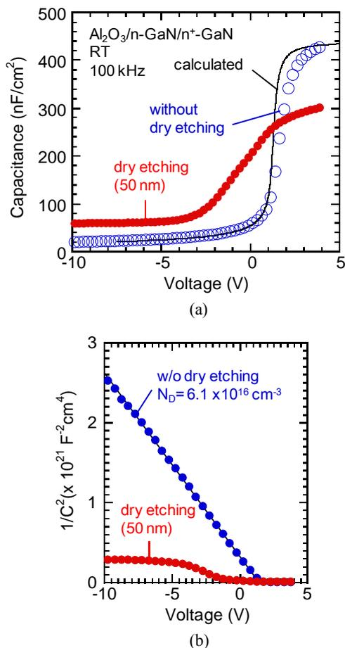
Fig.3 (a) C-V and (b)  $1/C^2$ -V plots of MOS samples with and without dry etching of AlGaIn surface.
