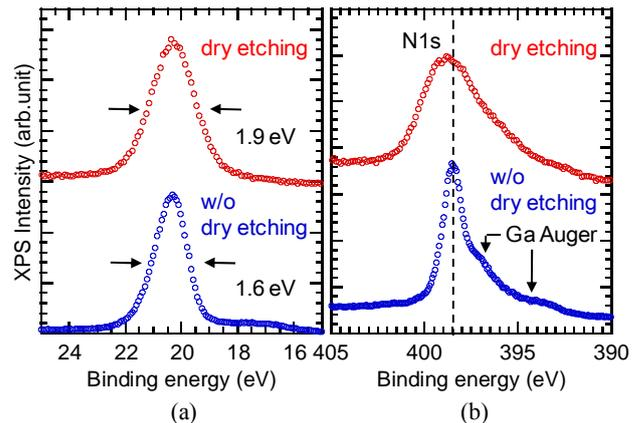
Fig.4 XPS spectra for (a) Ga3d and (b) N1s core levels from the GaN surfaces.
