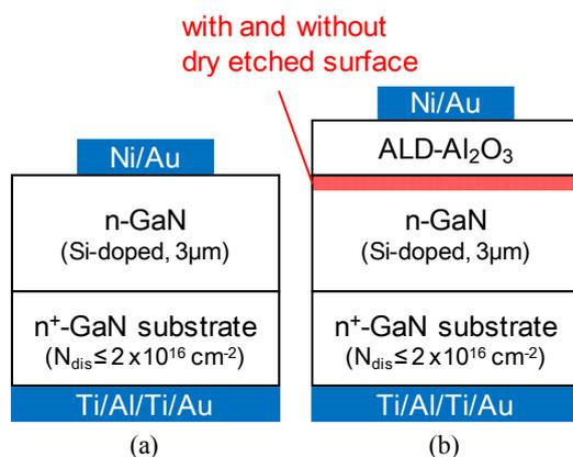
Fig.1 Sample structures for (a) Schottky and (b) MOS diodes.
