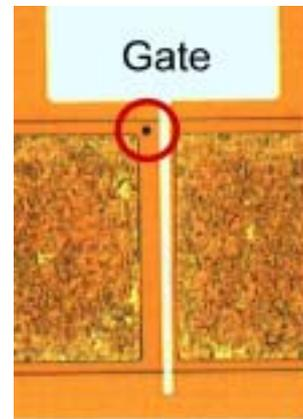
Fig. 4 Photo of the fabricated HEMT, where the defect is found (see the circled black dot).
