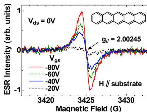
Fig. 1 First-derivative FI-ESR signals obtained with  $H$  parallel to the substrate. Inset shows chemical structure of pentacene.
