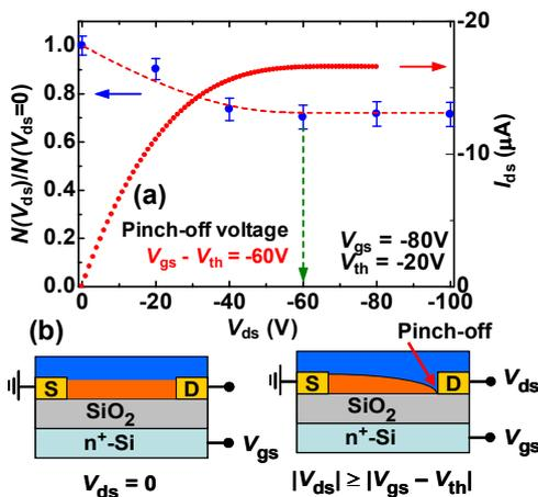
Fig. 2 (a)  $V_{ds}$  dependence of the carrier concentration ( $N$ ) normalized by the value at  $V_{gs} = 0$  together with the FET output current obtained for the same device. The gate voltage is  $-80$  V. Dashed curve represents the theoretical expectation using the potential distribution with  $\beta = 2.6$ . (b) Schematic illustration of charge carrier distribution within the channel.
