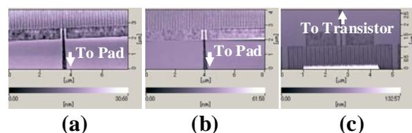
Fig.3 AFM images in the same position. (a) Sample A without wet treatment. (b) Sample A with wet treatment. (c) Sample B with wet treatment.
