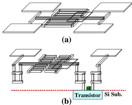
Fig. 1 Structure of test vehicle. (a) Sample A. (b) Sample B.
