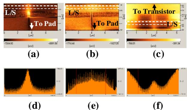
Fig.2 KFM images at the border of lines and spaces pattern. (a)(d) Sample A without wet treatment. (b)(e) Sample A with wet treatment. (c)(f) Sample B with wet treatment.
