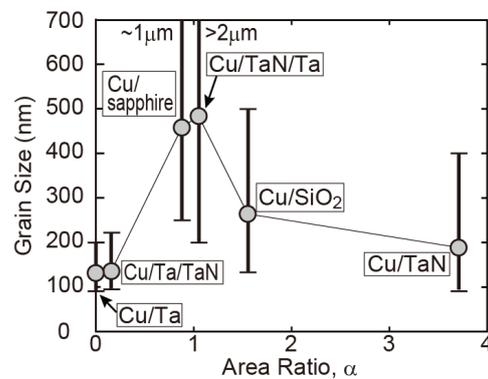
Fig. 5 The average Cu grain size of samples kept at RT after 150 days or more, as a function of the  $\alpha$  value.
