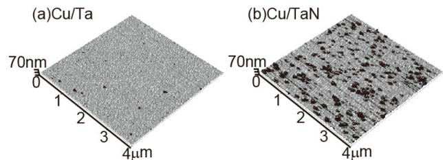
Fig. 6 AFM images of the (a) 10nm-Cu/Ta and (b) 10nm-Cu/TaN samples.
