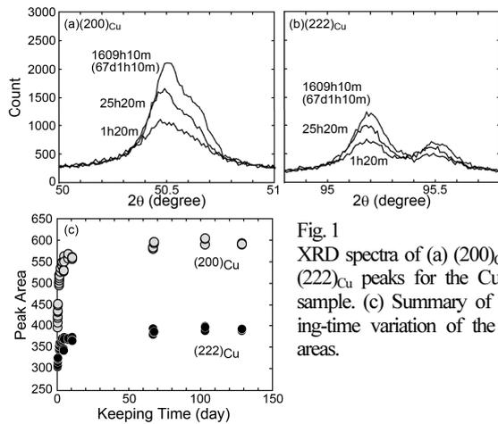
Fig. 1 XRD spectra of (a) (200)<sub>Cu</sub>, (b) (222)<sub>Cu</sub> peaks for the Cu/SiO<sub>2</sub> sample. (c) Summary of keeping-time variation of the peak areas.
