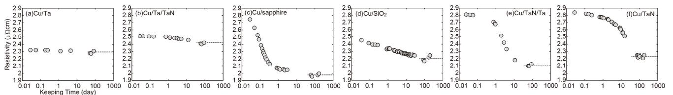
Fig. 3 The resistivity of the Cu films in (a) Cu/Ta, (b) Cu/Ta/TaN, (c) Cu/sapphire, (d) Cu/SiO<sub>2</sub>, (e) Cu/TaN/TaN, (f) Cu/TaN samples as a function of the keeping time.
