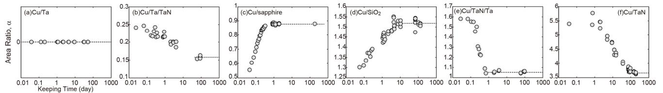
Fig. 2 The  $\alpha$  values for (a) Cu/Ta, (b) Cu/Ta/TaN, (c) Cu/sapphire, (d) Cu/SiO<sub>2</sub>, (e) Cu/TaN/TaN, (f) Cu/TaN samples as a function of the keeping time.
