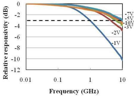
Fig. 4 Dependence of frequency response of MSM Ge-PD on dc bias voltage.
