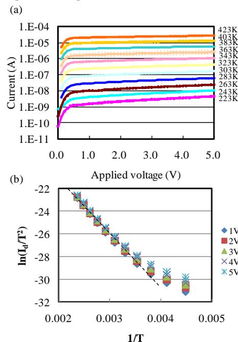
Fig. 3(a) Temperature dependence of dark current and (b) plotted data of  $\ln(I_d/T^2)$  vs.  $(1/T)$  with various bias voltages.
