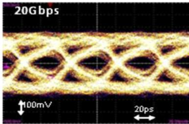
Fig. 5 Measured eye diagram at 20 Gbps with  $2^{15}$ -1 PRBS.
