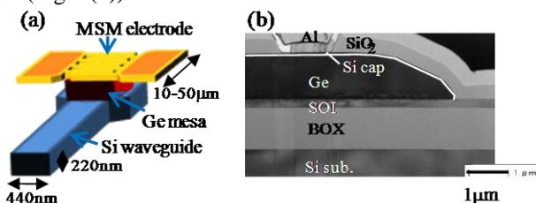
Fig. 1 (a) Schematic diagram and (b) cross-sectional TEM image of Si waveguide integrated MSM Ge-PD.
