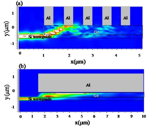
Fig. 6 Electric field density contour map of Si-waveguide coupled Ge-PD with Al electrode structure by 3D-FDTD method in case of (a) TM and (b) TE polarization light input.
