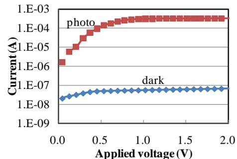
Fig. 2 Photoresponsivity of the fabricated MSM Ge-PD.
