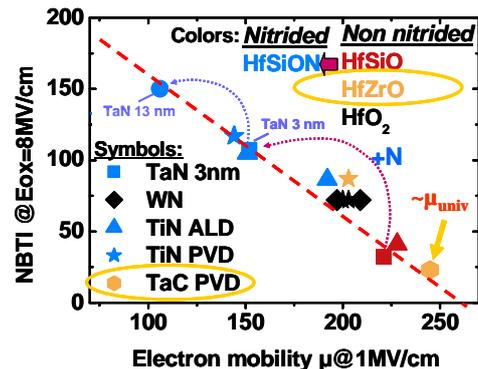
Fig.3: Correlation between PMOS NBTI and nMOS mobility for various gate stack compositions;  $\mu$  ( $\text{cm}^2/\text{Vs}$ ) measured at  $E=1\text{MV}/\text{cm}$ .
