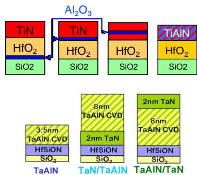
Fig.2: Main pMOS (Al-doped, Ti or Ta metal) stacks discussed in the paper. All devices are annealed at 1050°C.
