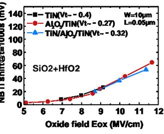
Fig.13: NBTI( $E_{ox}$ ). Splits on SiO2+HfO2:
