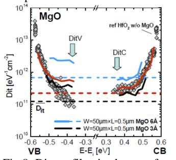
Fig.8: Dit profiles in the gap for various MgO thicknesses. MgO induces a states hump near the silicon valence band.
