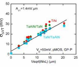
Fig.15:  $V_t$  mismatch for TaAlN gates compared to reference TiN / SOI (no doping).
