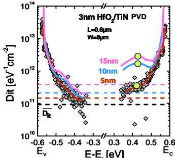
Fig.4: Effect of TiN thickness (5, 10, 15nm) on interface states profiles in the gap. N signature is a hump close to  $E_c$ .
