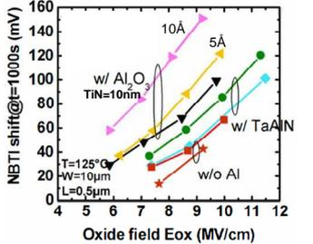
Fig.12: NBTI for various Al incorporation modes and compared to TiN references; stacks of Fig.2. SiO2 interface.
