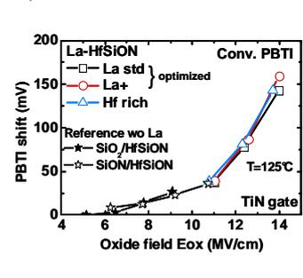
Fig.7: PBTI shift vs.  $E_{ox}$  for various optimized [La]. Neither PBTI dependence with La nor extra degradations are seen.
