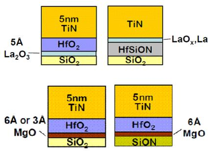
Fig.1: Main nMOS (La-doped or Mg-doped) stacks discussed in the paper. All devices are annealed at 1050°C.
