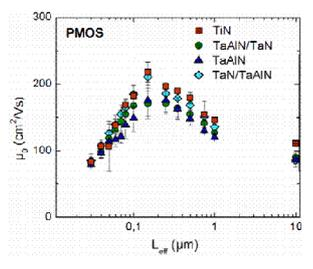
Fig.14: Low field hole mobility versus pMOS gate length (FDSOI). Good  $\mu$  is obtained for short channels.
