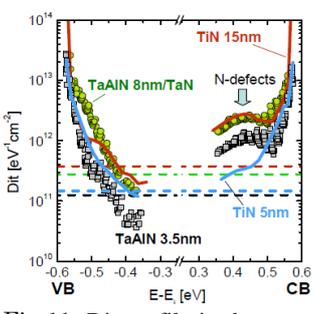
Fig.11: Dit profile in the gap with various stacks w/o Al. No specific Al signature is observed while N signature is enhanced.
