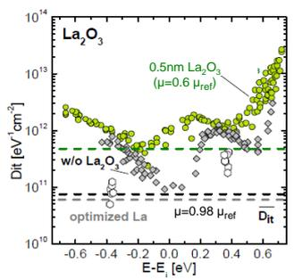
Fig.5: Dit(E) profiles in the gap with no\_La /high [La]/optimized\_La. Dash lines are mean values in the gap.
