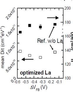
Fig.6: (■) Electron mobility and (□) Dit versus  $V_{fb}$  for various optimized La. Ref. without La is also given.
