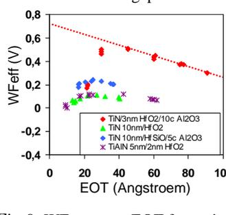
Fig.9:  $W_{Feff}$  versus EOT for various Al doping methods in the gate stack.  $W_{Feff}$  referred to Si mid-gap. SiO2 interface.
