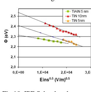
Fig.10: IPE Schottky plot at the metal gate side versus high-k electric field. TiAlN shows smaller barrier (more N+ behaviour) than TiN.
