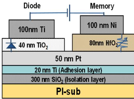
**Fig. 1** Schematic of a 1D1R cell by connecting an oxide diode of Ti/40nmTiO<sub>2</sub>/Pt, and a RS memory device of Ni/80nmHfO<sub>2</sub>/Pt in series.
