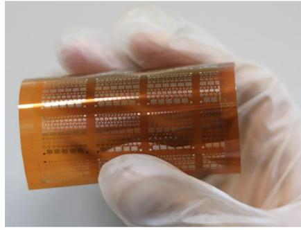
**Fig. 2** Photograph of fabricated flexible RS memory devices on a PI substrate.
