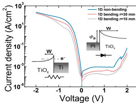
**Fig. 7** Rectifying characteristics of the Ti/40nmTiO<sub>2</sub>/Pt oxide diode with various bending curvatures.
