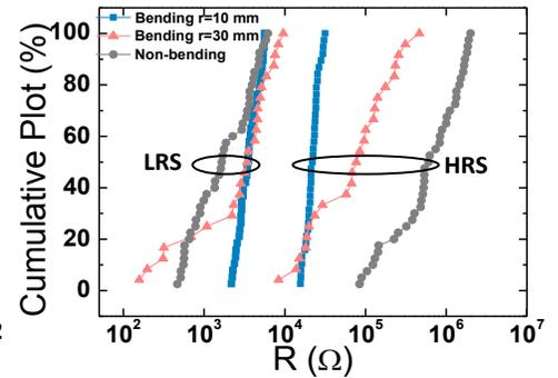
**Fig. 5** Cumulative percentages of LRS and HRS resistance of the Ni/80nmHfO<sub>2</sub>/Pt device with various bending curvatures.
