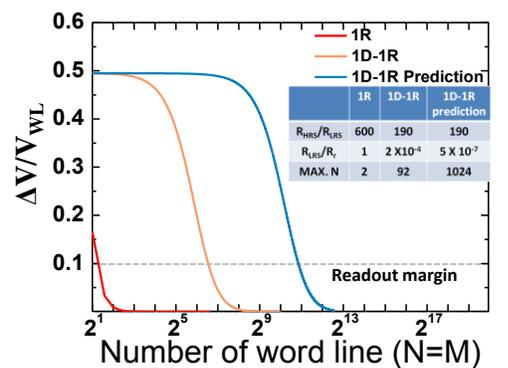
**Fig. 11** Calculated readout margin as a function of the number of word line in square ( $N=M$ ) crossbar 1R and 1D1R arrays.
