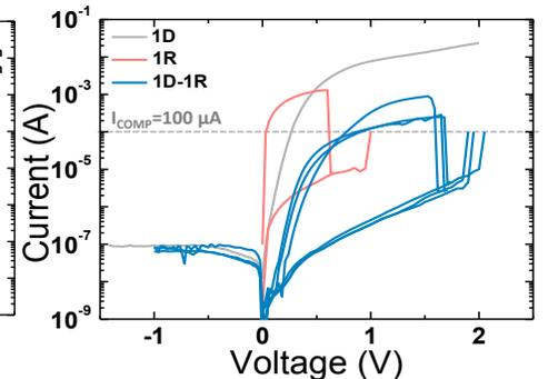
**Fig. 8** I-V characteristics of 1D, 1R and 1D1R in series.
