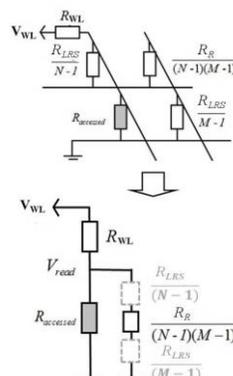
**Fig. 10** A simple equivalent circuit used to predict readout margin in a 1D1R crossbar memory array.
