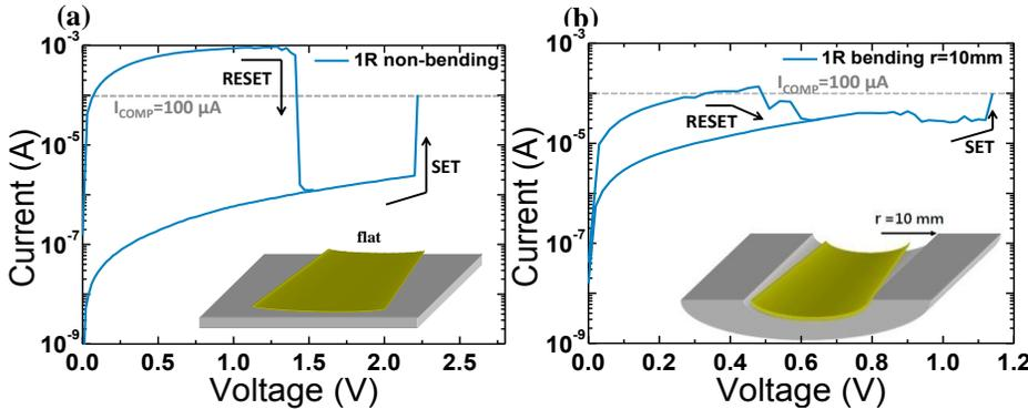
**Fig. 4** Unipolar RS characteristics of the Ni/80nmHfO<sub>2</sub>/Pt device at (a) flat, (b) bending ( $r=10$  mm) conditions.
