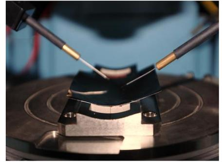
**Fig. 3** Photograph of electrical measurement setup and fabricated flexible RS memory devices under bending conditions.
