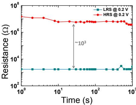
**Fig. 6** Read disturbance for HRS and LRS of the Ni/80nmHfO<sub>2</sub>/Pt device under constant stress (read) voltage of 0.2V.
