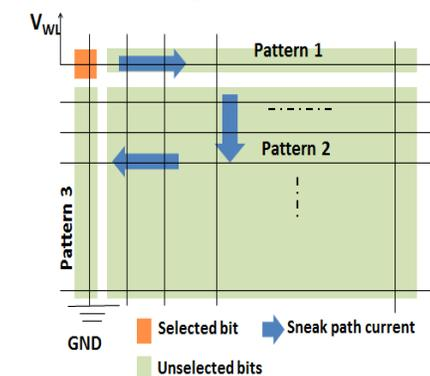
**Fig. 9** Schematic showing sneak paths through unselected bits at LRS during read in a crossbar memory array.
