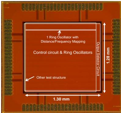
Fig. 1: Micrograph of the test chip
