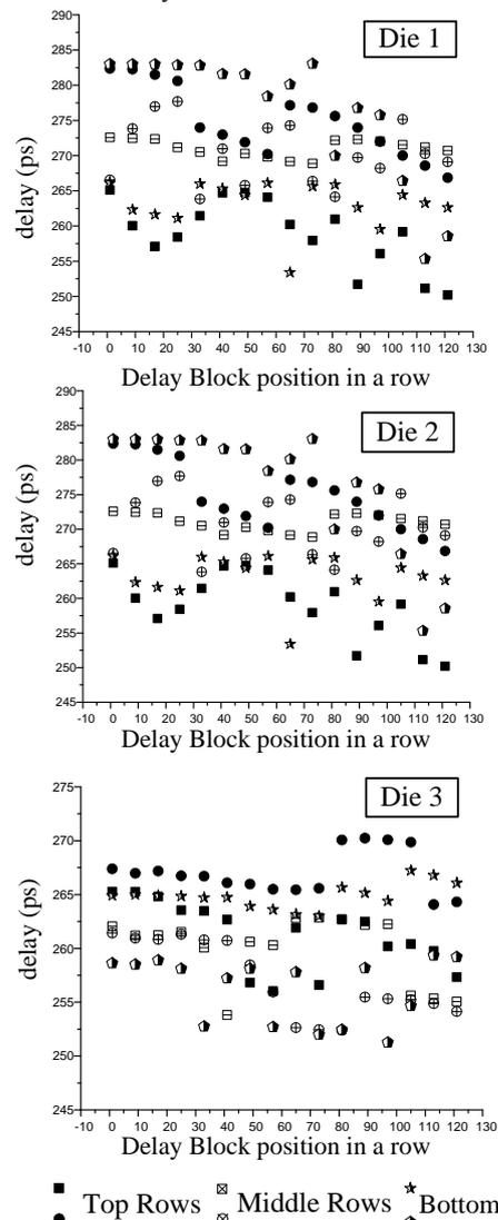
Fig. 3: Delay along different vertical position in a die
