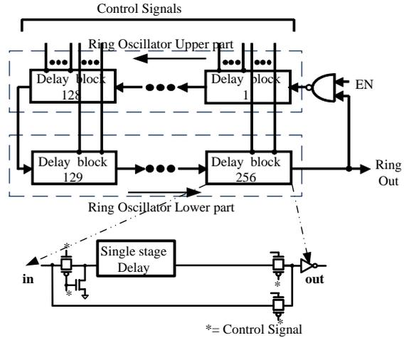
Fig. 2: Basic block diagram of a ring oscillator and detailed schematic of a delay block
