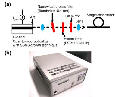
Figure 2 (a) Optical setup for wavelength tunable InAs/InGaAs QD-ECL using optical mode selection technique. (b) Compact bench-top coherent light source of developed narrow line-width wavelength tunable QD-ECL.
