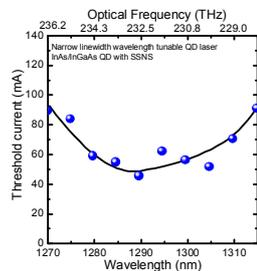
Figure 3 Dependence of threshold current on lasing wavelength of wavelength tunable InAs/InGaAs QD-ECL.
