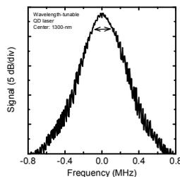
Figure 5 Estimation result for narrow line-width and stable operation of wavelength tunable InAs/InGaAs QD-ECL.
