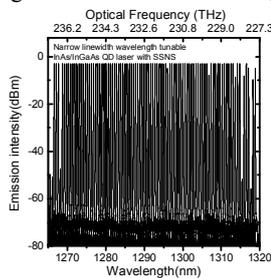
Figure 4 Ultra-broadband tuning-range of wavelength tunable InAs/InGaAs QD-ECL.
