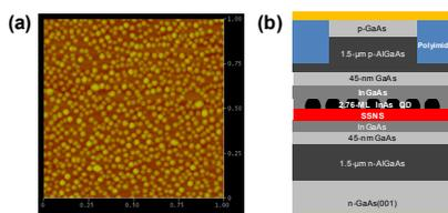
Figure 1 (a) AFM image of InAs/InGaAs QD structure fabricated using SSNS growth technique. (b) Cross-sectional image of ridge-type QD laser diode structure.
