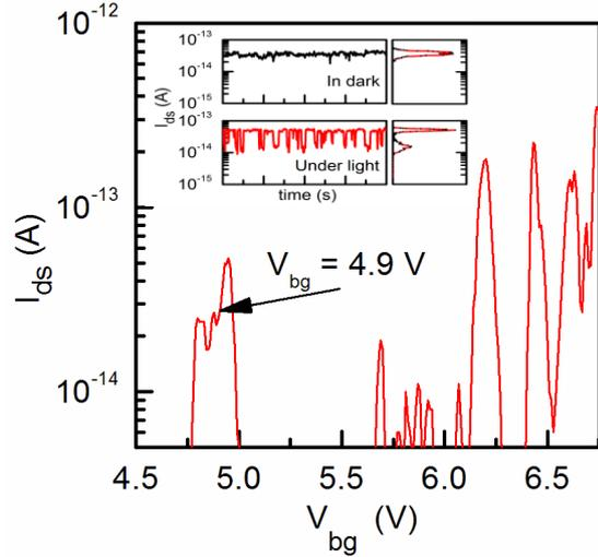
**Fig. 2.** Typical  $I_{ds}$ - $V_{bg}$  characteristics under light, showing current oscillation due to Coulomb blockade effect. (Inset)  $I_{ds}$ -time characteristics in dark and under light. Under light, current switches between two levels due to trapping of a photoelectron by a donor and subsequent detrapping.
