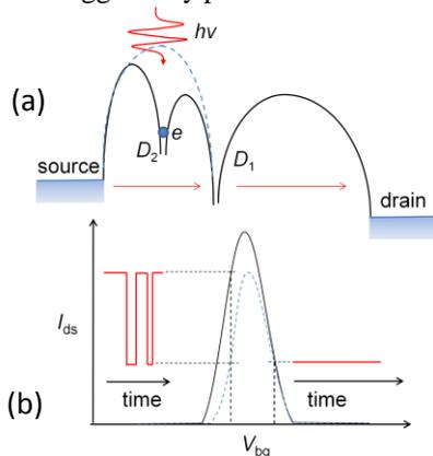
**Fig. 5.** (a) Illustration of the barrier height modulation due to trapping of a photoexcited electron by a trap donor ( $D_2$ ) sensed by single-electron tunneling via  $D_1$ . (b) Corresponding  $I_{ds}$ - $V_{bg}$  characteristics and RTS behavior for different  $V_{bg}$ .
