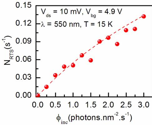
**Fig. 3.** Number of RTS versus incident photon flux ( $\phi_{inc}$ ), showing an increasing dependence, indicating that RTS is triggered by photons.
