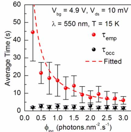
**Fig. 4.** Average time of empty ( $\tau_{emp}$ ) and occupied ( $\tau_{occ}$ ) states of the trap versus incident photon flux ( $\phi_{inc}$ ).
