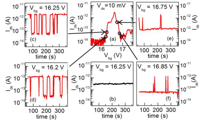
**Fig. 6.** (a) First peak of  $I_{ds}$ - $V_{bg}$  characteristics. (b)  $I_{ds}$ -time characteristics in dark. (c)-(f)  $I_{ds}$ -time characteristics under light for  $V_{bg}$  on the left side of peak [(c) and (d)] and on the right side [(e) and (f)].
