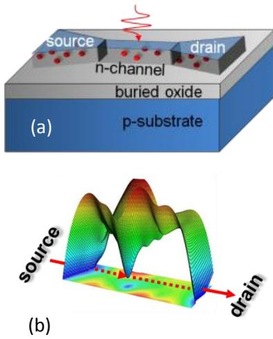
**Fig. 1.** (a) Schematic SOI-FET device structure. (b) Single-electron transport through a single donor.
