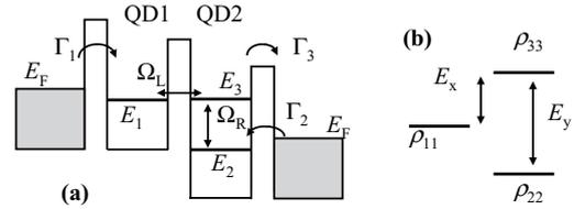
FIG. 1: (a) A three-level system in double QDs (DQDs). A bias voltage is applied between the left and right electrodes. (b) A density matrix for the three level. We define  $E_x \equiv E_3 - E_1$  and  $E_y \equiv E_3 - E_2$ . The dark state is a state with  $\rho_{33} = 0$ .
