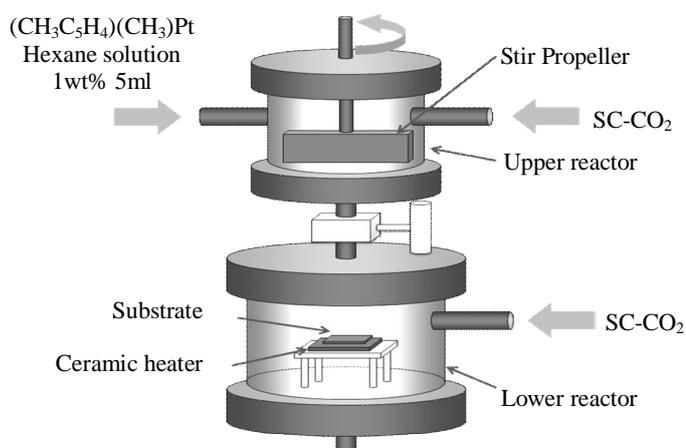
Fig. 2 Schematic of SCF-CVD system used for the preparation of Pt nanoparticles.
