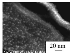
Fig. 5 SEM image of Pt-supported CNW on carbon fiber paper.
