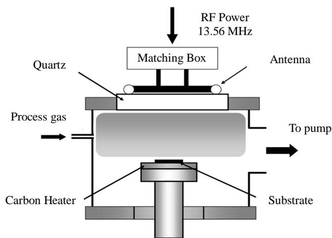
Fig. 1 Schematic of ICP system used for the growth of CNWs.
