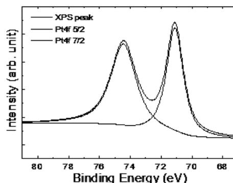
Fig. 6 XPS spectrum of Pt-supported CNW after SCF-MOCVD.
