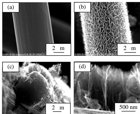
Fig. 3 (a) SEM image of carbon fiber forming paper structure. (b)(d) SEM images of CNWs grown on carbon fiber.
