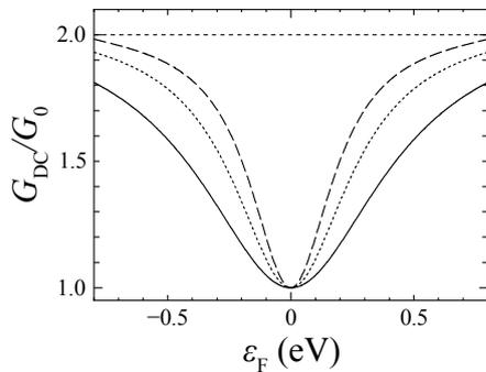
Fig. 1. Fermi-level dependence of the DC conductance of armchair SWNTs with a single atomic vacancy. Solid, dotted, and dashed lines show the DC conductance behaviors of (6,6), (8,8), and (10,10) SWNTs with a single atomic vacancy, respectively, and short-dashed line shows that of pristine armchair SWNTs.  $G_0$  is the quantum conductance unit.
