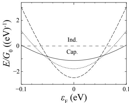
Fig. 2. Fermi-level dependence of the emittance in armchair SWNTs with a single atomic vacancy. Solid, dotted, and dashed lines show the emittance behaviors of (6,6), (8,8), and (10,10) SWNTs with a single atomic vacancy, respectively.
