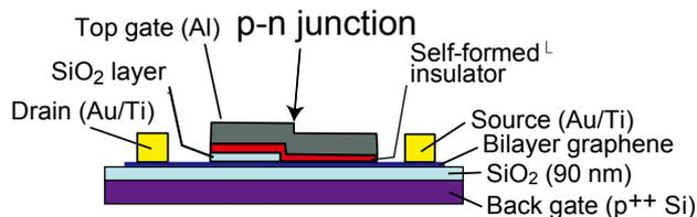
Fig. 1. Schematic draw of a graphene  $p$ - $n$  junction controlled by stepwise top gate. The bottom surface of Al (top gate) electrode is naturally oxidized and insulates the top gate from the graphene [4]. The stepwise top gate structure is made by an additional SiO<sub>2</sub> layer which covers the graphene channel partly.
