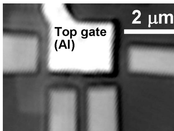
Fig. 3. Laser microscope image of a bilayer graphene  $p$ - $n$  junction. An Al top gate is deposited on the structure in the Fig. 2.
