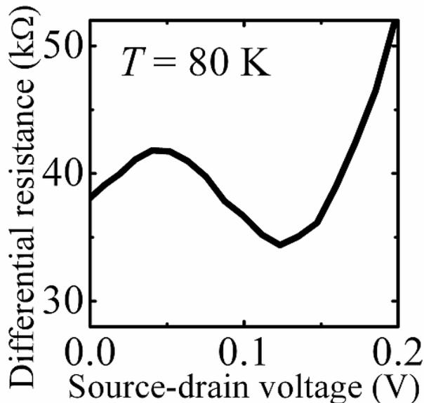
Fig.4. Differential resistance as a function of the source-drain voltage.
