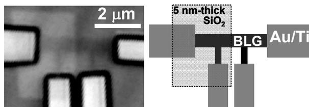
Fig. 2. Laser microscope image (left) and schematic draw of bilayer graphene covered partially by 5 nm-thick SiO<sub>2</sub>. The graphene is patterned by oxygen plasma and contacted by Au/Ti electrodes for four-terminal measurement, followed by the SiO<sub>2</sub> deposition.
