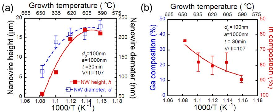
**Fig. 2:** Temperature dependence of nanowire (a) height,  $h$ , and diameter,  $d$ , and (b) composition. The error bar in (a) shows maximum & minimum and in (b) shows FWHM, respectively.
