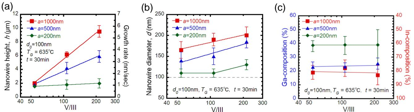
**Fig. 3:** V/III ratio dependence of nanowire (a) height,  $h$ , (b) diameter,  $d$ , and (c) composition. The dashed line of inset (b) shows  $d_0$ . The error bar in (a),(b) shows maximum & minimum and in (c) shows FWHM, respectively.
