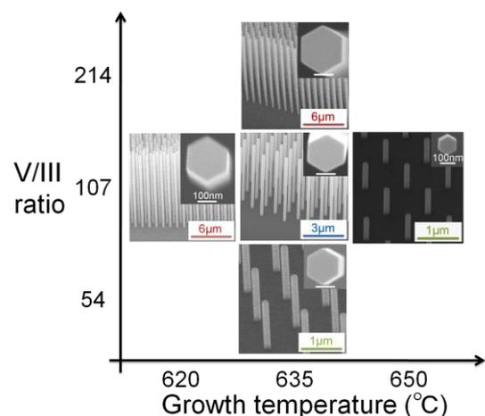
**Fig. 1:** 45° tilted SEM images of InGaAs NWs grown at different  $T_G$  and V/III ratio. Inset shows a top view of the NW. The opening pitch,  $a$ , was 1000 nm, respectively. White scale bar : 100nm.
