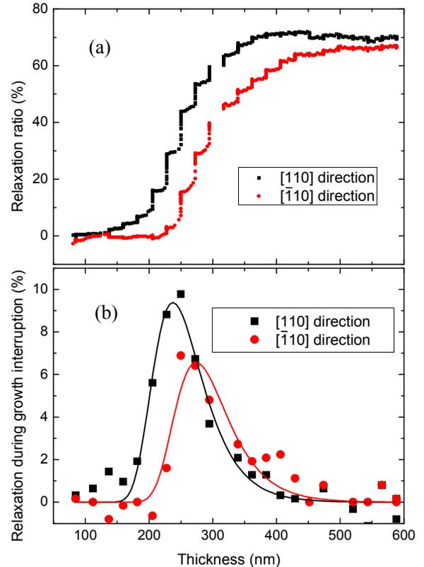
Fig. 3 Film thickness dependence on the degree of relaxation for  $\text{In}_{0.08}\text{Ga}_{0.92}\text{As}$  film (a) and that during growth interruptions (b).
