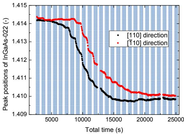
Fig. 2 Time evolution of peak positions for the InGaAs 022 peak along [110] and  $[\bar{1}\bar{1}0]$  directions. The white and blue bands indicate periods of crystal growth and growth interruption, respectively.
