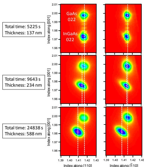
Fig. 1 Typical *in situ* RSM for 022 diffractions after measuring for 5225, 9643 and 24838 sec, corresponding to the  $\text{In}_{0.08}\text{Ga}_{0.92}\text{As}$  film thicknesses of 137, 234 and 588 nm, respectively.
