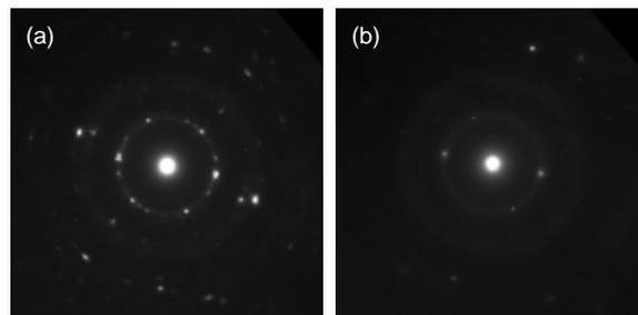
Fig. 5 Electron diffraction patterns of FLC poly-Ge observed at positions (a) and (b) indicated in Fig. 4.
