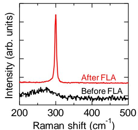
Fig. 2 Raman spectra of Ge films before and after FLA.
