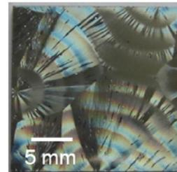
Fig. 1 Surface of a FLC poly-Ge film.
