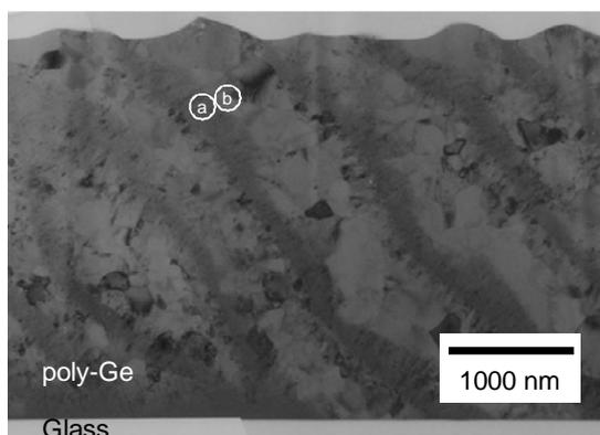
Fig. 4 Cross-sectional TEM image of a FLC poly-Ge film. The cross-section was formed along a crystallization direction.
