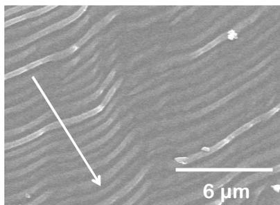
Fig. 3 Surface SEM image of a FLC poly-Ge film. An arrow indicates a lateral crystallization direction.
