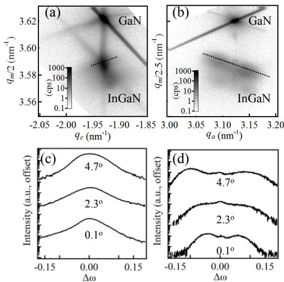
Fig. 1 RSMs of (a)  $(20\bar{2}1)$  and (b)  $(21\bar{3}0)$  diffractions from group-B InGaN film on  $0.1^\circ$ -off GaN substrate. Rocking curves for InGaN (c)  $(20\bar{2}1)$  and (d)  $(21\bar{3}0)$  diffraction.
