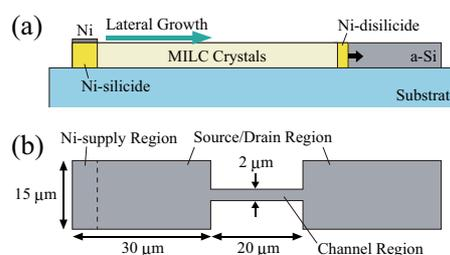
**Fig. 1:** (a) Schematic illustration of MILC process (cross section). Slices of nickel di-silicide move towards a-Si leaving epitaxial silicon behind. (b) Layout of the patterned a-Si film and the position of Ni to induce MILC.
